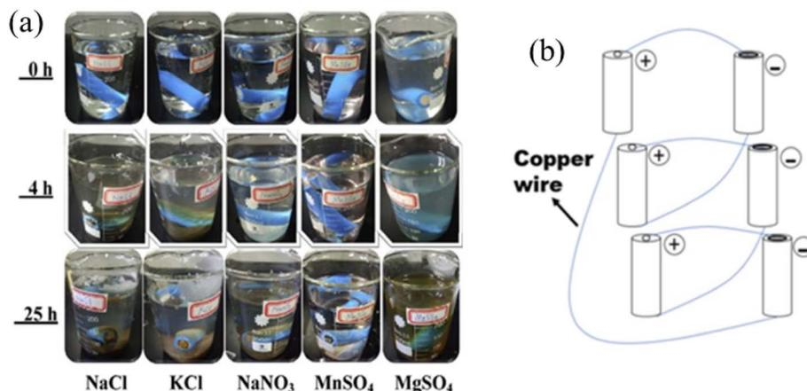
Fig. 1 (a) Discharging process using different salts to promote short-circuiting by removing remaining electricity.<sup>31</sup> (b) Discharging process using copper wire.<sup>12</sup>
