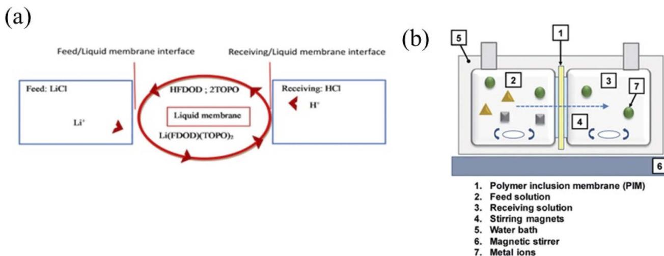
Fig. 2 (a) Scheme of the mechanism of transport using a supported liquid membrane (modified based on ref 92); (b) schematic diagram of the polymer inclusion membrane transport cell.<sup>91</sup>
