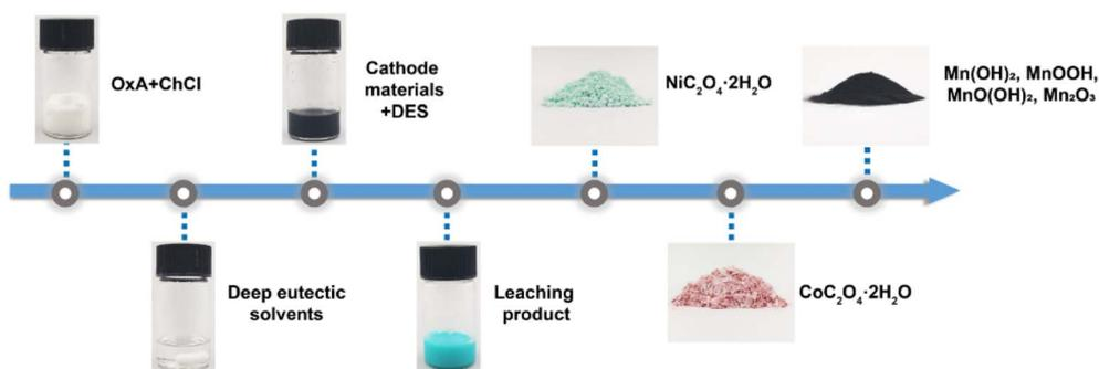
Fig. 3 Flow chart for DES-based separation of Ni, Co, and Mn from exhausted LIBs.<sup>107</sup>
