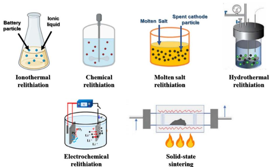
Fig. 5 The different technologies used in the direct regeneration processes (modified based on ref 80,137,140).
