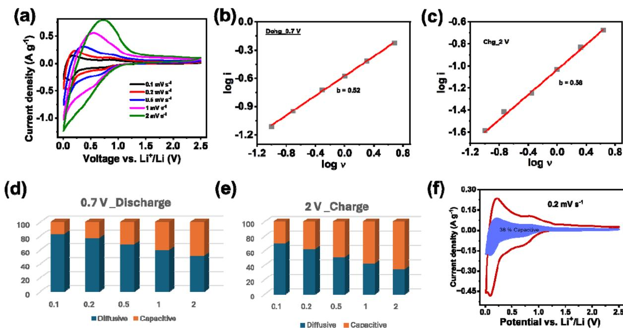
Fig. 5 (a) CV at various scan rates of 0.1, 0.2, 0.5, 1, and  $2 \text{ mV s}^{-1}$ ;  $\log i'$  vs.  $\log v'$  plot (b) at cathodic peak 0.7 V, (c) at anodic peak 2 V; (d) capacitive and diffusive percentage at various scan rates corresponding to (d) 0.7 V peak, (e) 2 V peak; (f) the capacitive contribution to the total charge storage at  $0.2 \text{ mV s}^{-1}$ , for CF-mCO-R half-cell.
