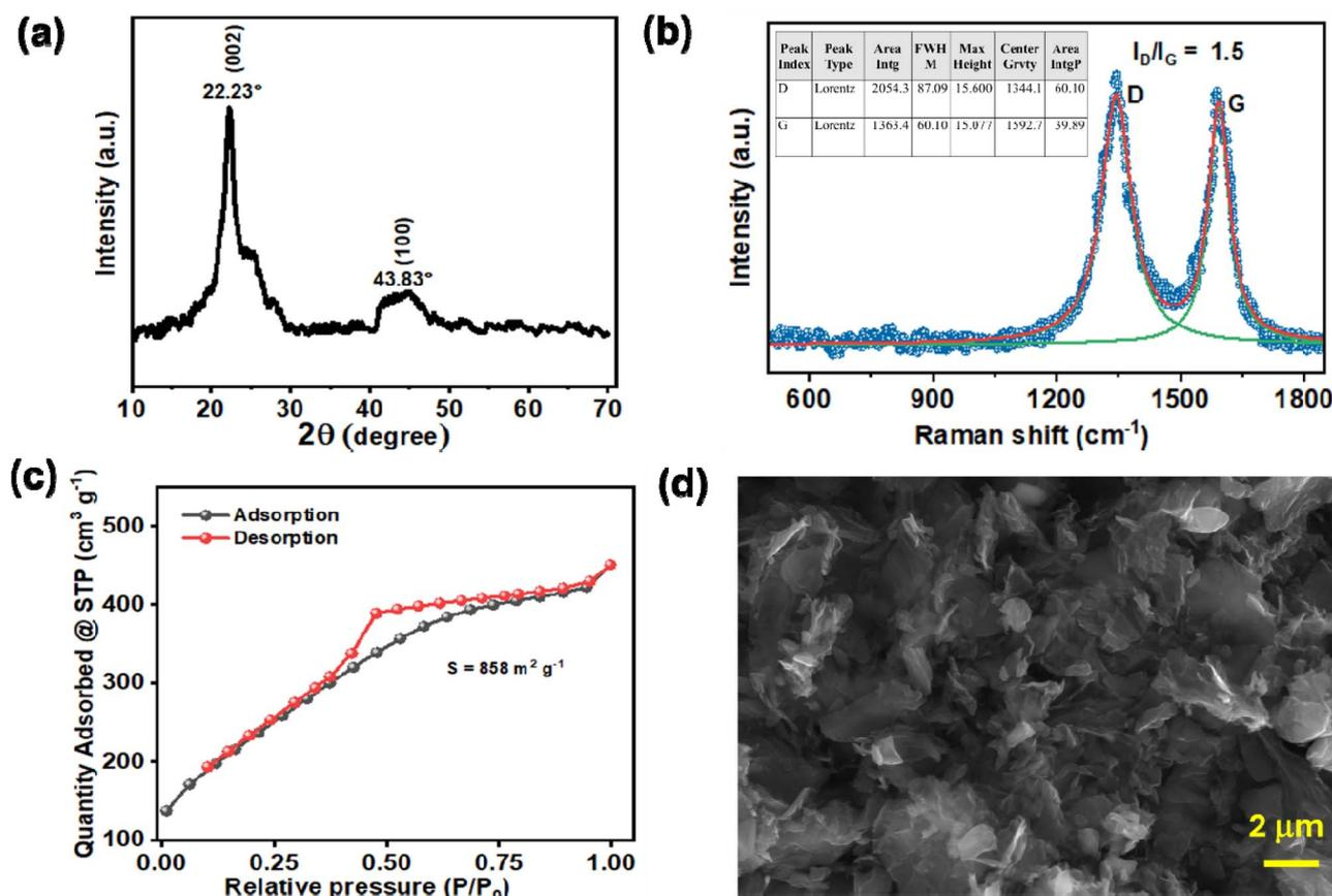
Fig. 1 (a) XRD diffractometer, (b) Raman spectra, (c) N<sub>2</sub>-adsorption–desorption isotherm, (d) SEM images of AGO-R materials.
