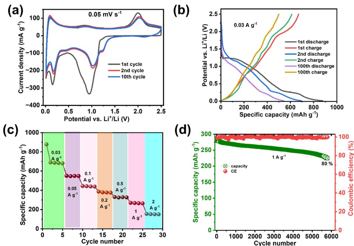
Fig. 4 (a) Cyclic voltammogram at  $0.05 \text{ mV s}^{-1}$ , (b) GCD profile at  $0.03 \text{ A g}^{-1}$ , (c) C-rate studies at various current densities of 0.03, 0.05, 0.1, 0.2, 0.5, 1, and  $2 \text{ A g}^{-1}$ , (d) cycling stability plot with coulombic efficiency at  $1 \text{ A g}^{-1}$ , of in the voltage range of 0.01 to 2.5 V for CF-mCO-R half-cell.
