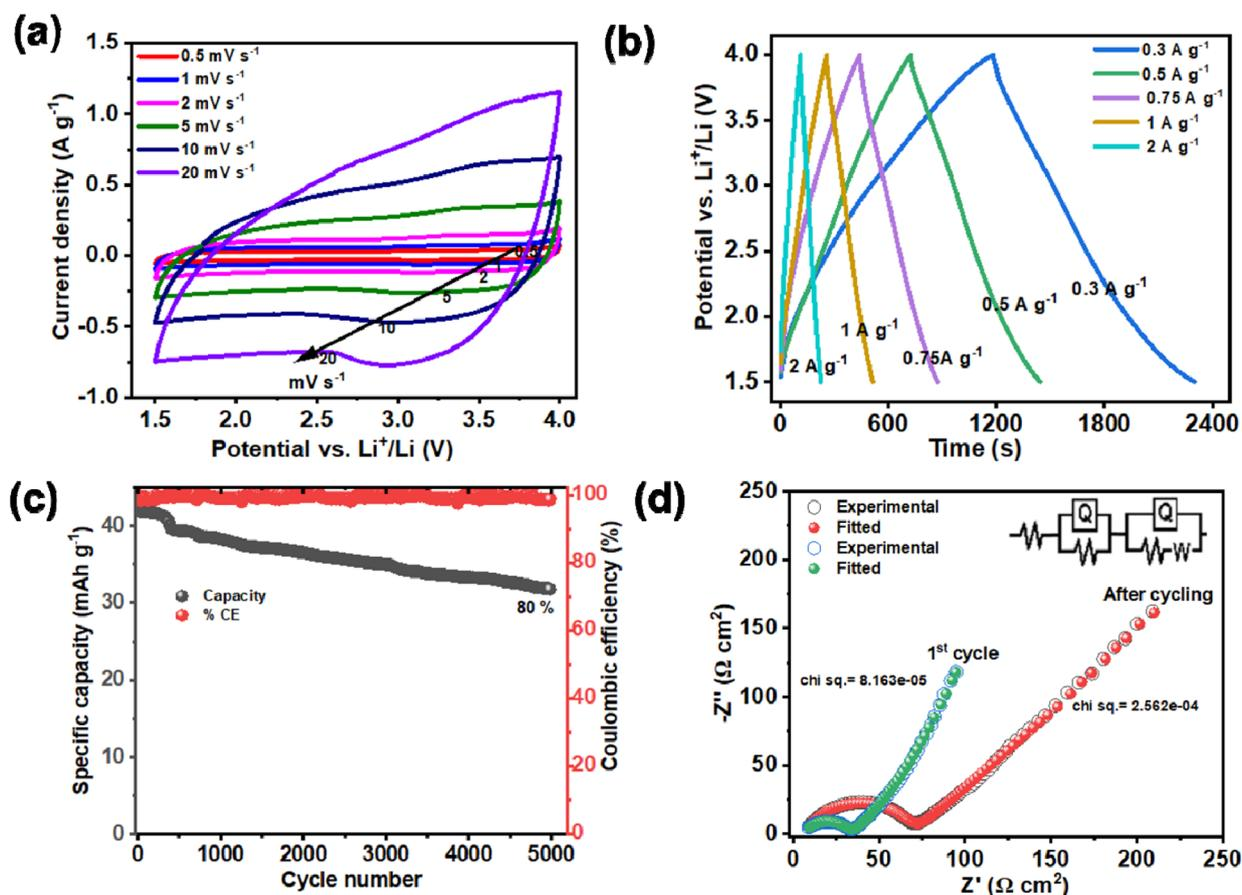
Fig. 3 (a) Cyclic voltammogram, (b) voltage profile, (c) cycling stability, (d) EIS spectra and equivalent circuit model (inset) for the CF-AGO-R cathode half-cell vs.  $\text{Li}^+/\text{Li}$ .
