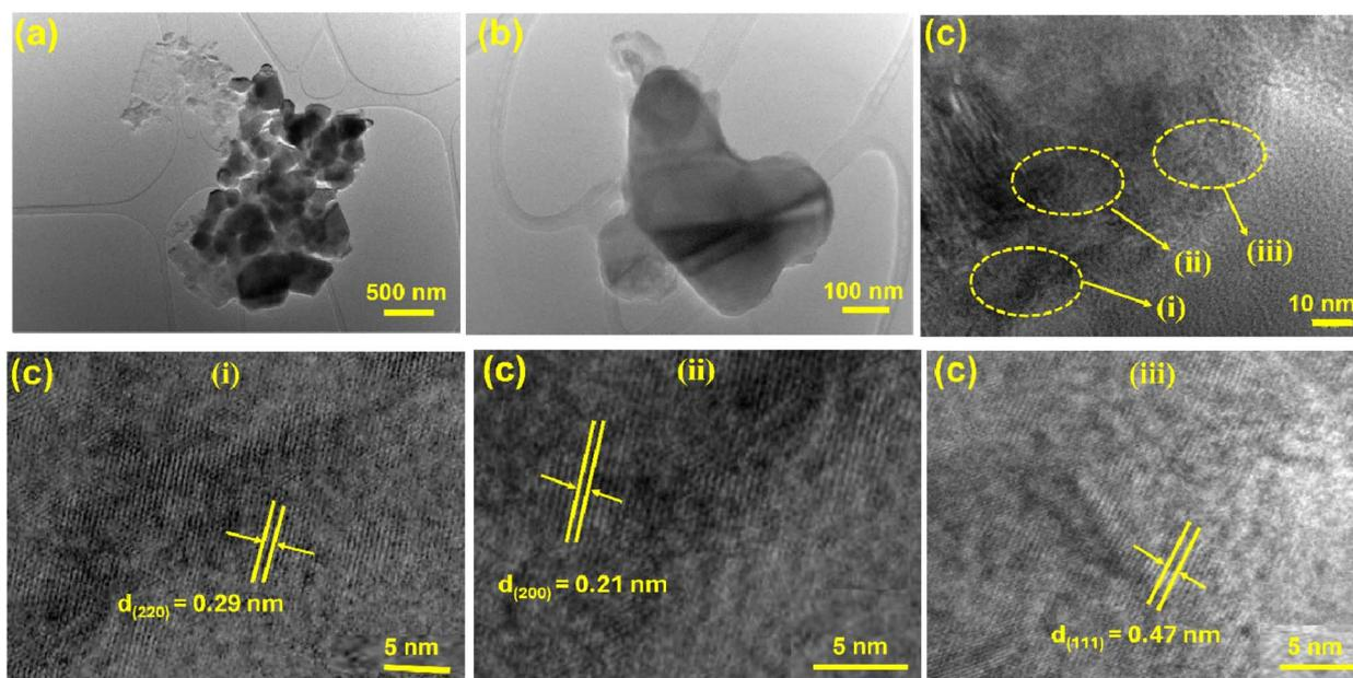
Fig. 2 (a) Low magnification TEM image, (b) TEM micrograph of a single particle, (c) different lattice fringes, (c-i)  $d = 0.29 \text{ nm}$  corresponding to (220) of  $\text{Co}_3\text{O}_4$ , (c-ii)  $d = 0.21 \text{ nm}$  corresponding to (200) plane of CoO, and (c-iii)  $d = 0.47 \text{ nm}$  (111) plane of  $\text{Co}_3\text{O}_4$  crystal, of mCO-R materials.
