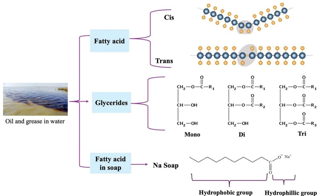
Fig. 3 Major components in FOG deposition and their chemical structure. Image source: Oil spill photo – Jesse Kavanaugh, U.S. Coast Guard.
