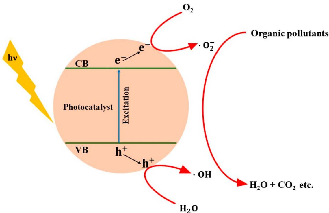
Fig. 16 Photocatalytic oxidation process mechanism.<sup>166</sup>
