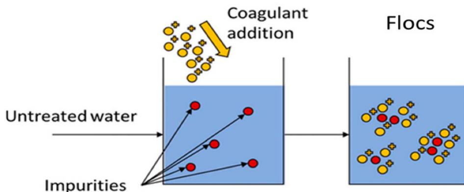
Fig. 10 Coagulation/flocculation mechanisms.<sup>104</sup>
