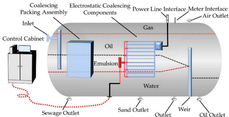
Fig. 8 Gravity separation tank.<sup>91</sup>
