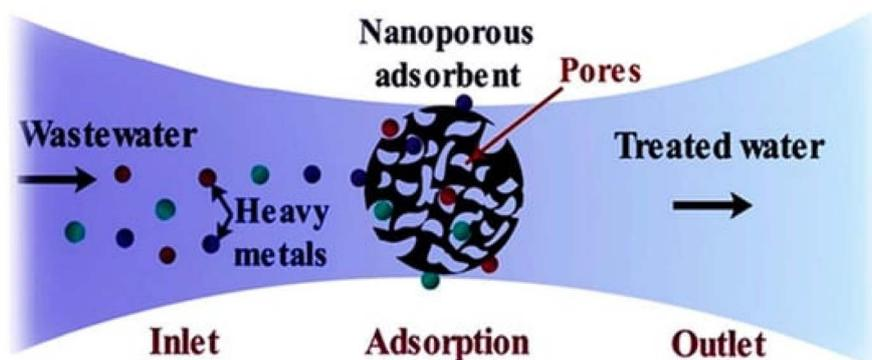
Fig. 13 Adsorption of heavy metals by a nanoporous adsorbent.<sup>120</sup>
