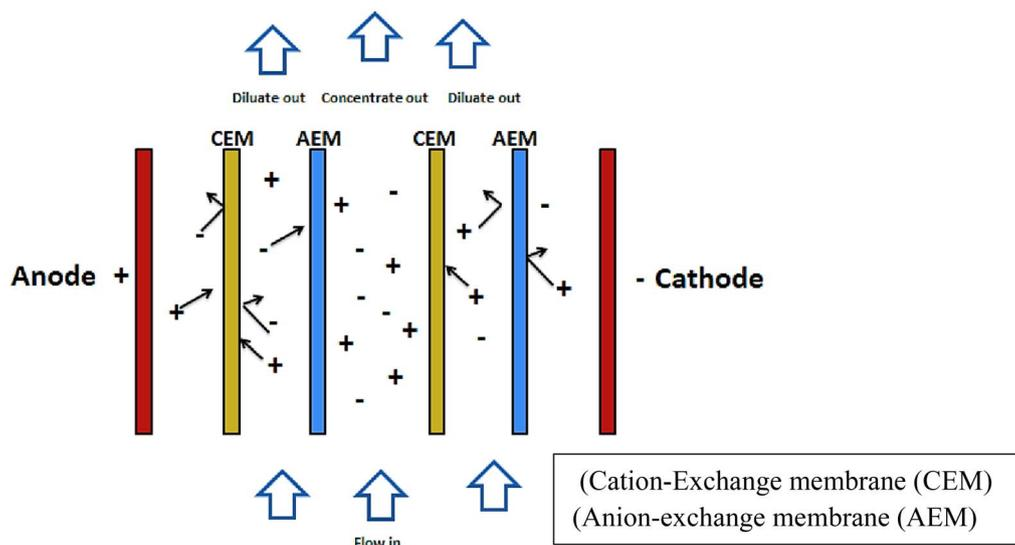
Fig. 14 Electrodialysis.<sup>139</sup>
