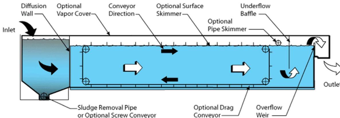
Fig. 11 API oil–water separator.<sup>107</sup>
