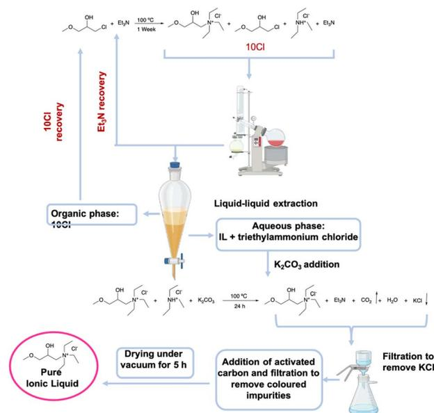
Scheme 3 Purification process of [N<sub>2</sub>O*R*]Cl ionic liquids.
