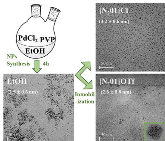
Fig. 14 TEM Images of Pd NPs in ethanol, [N<sub>2</sub>O1]Cl and [N<sub>2</sub>O1]OTf.
