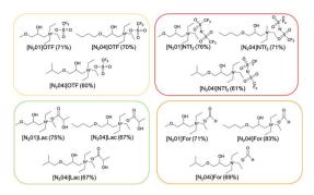
Fig. 4 Structures and isolated yields of glycerol-derived ionic liquids synthesized by ion-exchange reactions from chlorides.
