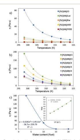
Fig. 8 Dynamic viscosities of glycerol-derived [N<sub>2</sub>OR]X ILs for different (a) anions, (b) R-chains, and (c) water content in [N201]CL
