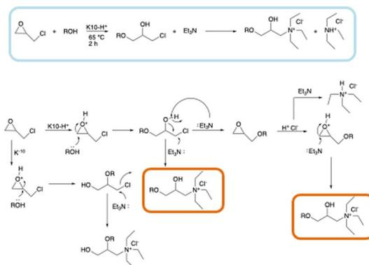
Scheme 2 Reaction pathways for the synthesis of ionic liquids from epichlorohydrin.
