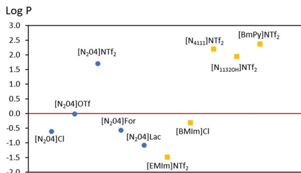
Fig. 10 Comparison of  $\log P$  values of  $[\text{N}_2\text{O}4]\text{X}$  ILs (this work) with some values examples from the literature.<sup>48,49</sup>
