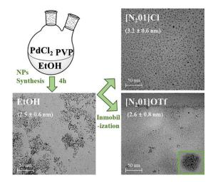
Fig. 14 TEM Images of Pd NPs in ethanol, [N<sub>2</sub>01]Cl and [N<sub>2</sub>01]OTf.
