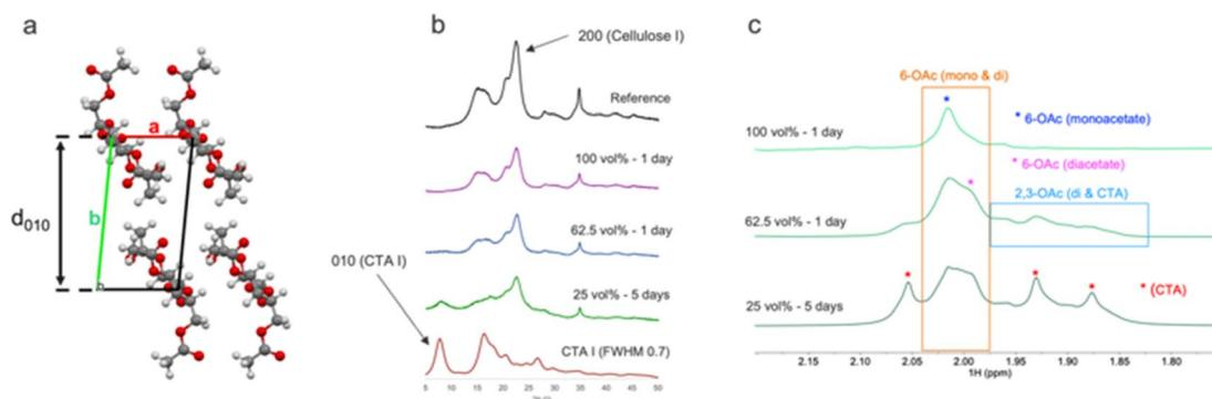
Fig. 6 Appearance of the CTA I (010) X-ray diffraction plane, in WAXS concomitant with CTA formation from comparison with NMR. (a) CTA I crystal structure with the (010)  $d$ -spacing highlighted. (b) Comparison of the experimental WAXS samples with a calculated diffraction pattern for CTA I (FWHM of 0.7). (c) Assigned acetate region in the diffusion-edited  $^1\text{H}$  NMR spectra.
