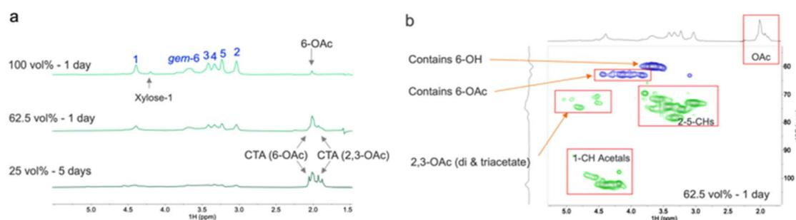
Fig. 2 Regioselectivity of the representative samples through solution-state NMR analysis. (a) Diffusion-edited  $^1\text{H}$  NMR analysis showing the 2,3,6-OAc regioselectivity pattern in the acetate region (2 ppm), (b) multiplicity-edited HSQC spectrum for one of the key samples, as an additional method of confirming the regioselectivity.
