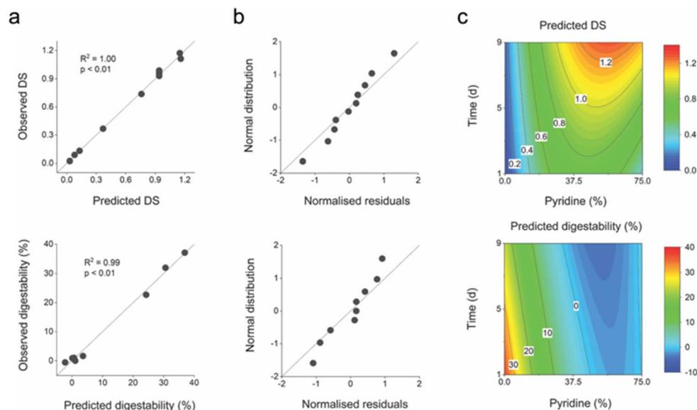
Fig. 10 Response surfaces for acetylation DS and enzymatic digestibility. (a) Observed vs. predicted properties. (b) Normalised model residuals. (c) Predicted response surfaces, linking reaction time and  $\text{Ac}_2\text{O}:\text{Pyr}$  vol% ratios, to the degree of substitution (above) and enzymatic digestibility (below).
