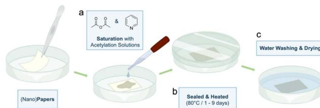
Fig. 1 Laboratory procedure for acetylation of the (nano)paper hand sheets. The individual steps involve (a) saturation with the acylation solution. (b) ‘Ripening’ (heating) for the appropriate time. (c) Final washing and drying.
