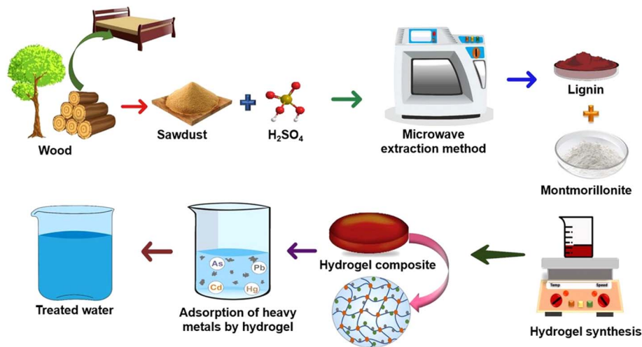
Fig. 8 A schematic overview of the preparation of a lignin–montmorillonite composite hydrogel and the adsorption of heavy metals [reproduced from ref. 249 with permission from American Chemical Society, Copyright 2024].
