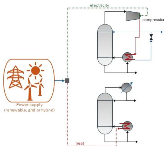
Fig. 5 Heat pump assisted distillation with MVR.
