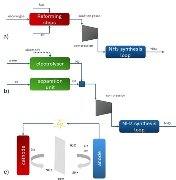
Fig. 1 Haber–Bosch process, (a) conventional, (b) indirectly electrified and (c) directly electrified.
