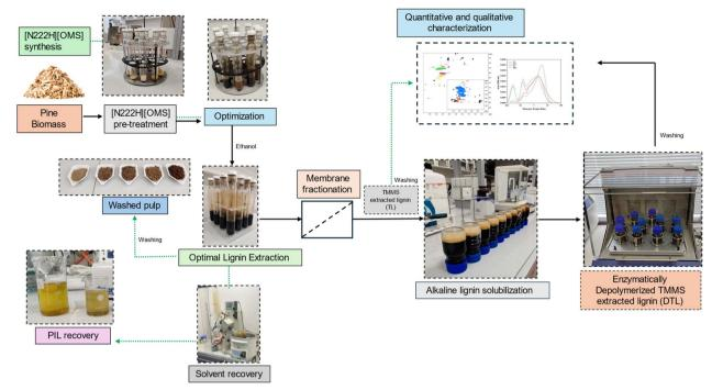
Overview of the lignin extraction and its depolymerization process from PWB biomass using [N222H][OMS] PIL
