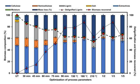
Fig. 2 Optimization of the lignin extraction process from PWB using [N222H][OMs] PIL, focusing on three key parameters: process time, temperature and biomass loading to PIL ratio.
