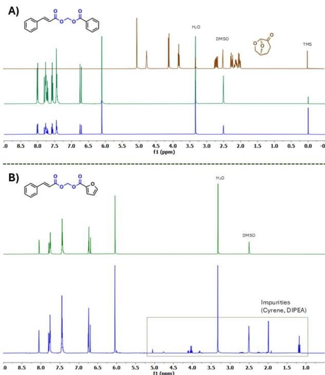
Fig. 6 Stacked <sup>1</sup>H-NMR spectra (DMSO-*d*<sub>6</sub>, 400 MHz) of (A) acylal **8c** after precipitation (blue) and DCPC (green). Here, no remains of starting material, Cyrene (brown spectra as reference) or DIPEA are detectable. (B) Precipitated solid of acylal **8b** (blue) contains significant amounts of Cyrene and DIPEA. DCPC purification is required and leads to pure compound (green).
