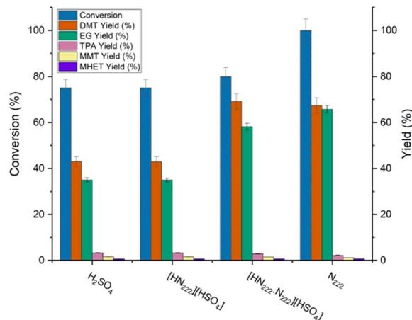
**Fig. 2** Conversion (%) of PET and the yield (%) of DMT using a variation of catalysts ranging from acidic to basic. Reaction conditions: PET (0.002 mol), catalysts (0.01 mol), methanol (0.15 mol) and a reaction temperature of 180 °C for 1 h. All reactions were carried out in triplicate.
