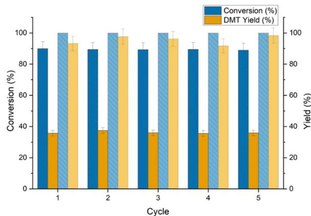
Fig. 6 The reusability cycle of  $[\text{HN}_{222}\cdot\text{N}_{222}][\text{HSO}_4]$  on the conversion (%) and DMT yield (%). Reaction conditions: PET (0.005 mol)  $[\text{HN}_{222}\cdot\text{N}_{222}][\text{HSO}_4]$  (0.01 mol), methanol (0.15 mol) (dark blue and orange). PET (0.0025 mol)  $[\text{HN}_{222}\cdot\text{N}_{222}][\text{HSO}_4]$  (0.01 mol), methanol (0.15 mol) (light blue and orange) and a reaction temperature of 180 °C for 3 h.
