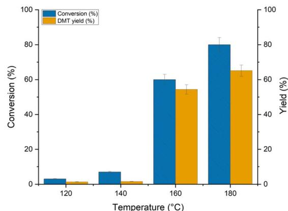
**Fig. 3** Effect of temperature on conversion (%) and DMT yield (%). Reaction conditions: PET (0.002 mol) [HN<sub>222</sub>·N<sub>222</sub>][HSO<sub>4</sub>] (0.01 mol), methanol (0.15 mol) and a reaction temperature of 120–180 °C for 1 h. All reactions were carried out in triplicate.
