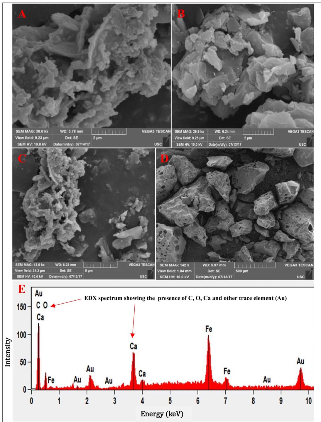
Fig. 4 (A–E) SEM micrographs and accompanying EDX elemental analysis illustrating the morphology of the MNP hydrochar obtained after 6 h of HTC. The images were captured at view fields of 9.23 μm, 9.25 μm, 21.3 μm, and 1.94 mm, highlighting the MNP hydrochar's aggregated microstructure and elemental composition.
