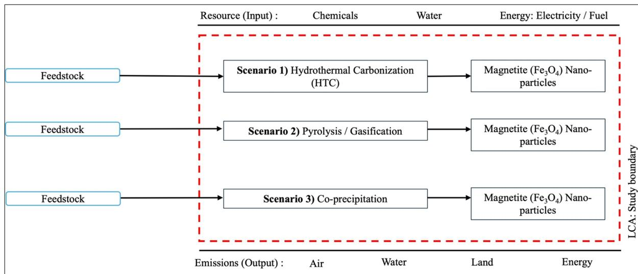
Fig. 2 System boundary for the LCA of magnetite ( $\text{Fe}_3\text{O}_4$ ) nanoparticle (MNP) production via three pathways: (1) hydrothermal carbonization (HTC), (2) pyrolysis/gasification, and (3) co-precipitation. The red dashed box delineates the LCA study boundary, encompassing resource inputs (chemicals, water, and energy) and emissions outputs (air, water, land, and energy). Blue-outlined rectangles represent the feedstock input streams for each scenario.
