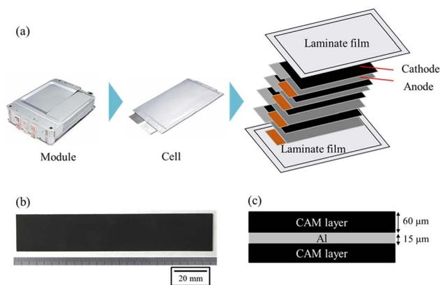
Fig. 1 Schematic of LiB cathode sheet sample. (a) Structure of the laminated LiB, (b) top view of the extracted cathode sheet, and (c) cross-sectional schematic of the cathode sheet.
