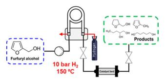
Scheme 2 Schematic of Flowsyn continuous flow reactor for the liquid phase catalytic hydrogenation of FALC to 1,5-PeD in toluene.
