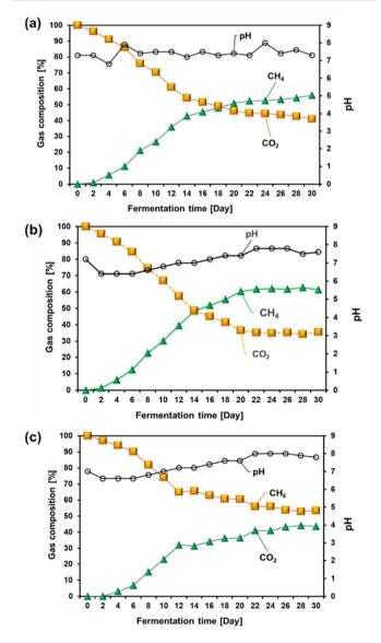
Fig. 3 Effect of algae-to-cow manure ratio on gas composition during the acclimatization process: algae-to-cow manure ratios of (a) 1:1, (b) 2:1, and (c) 3:1.
