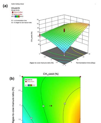
Fig. 9 (a) Three-dimensional surface and (b) contour plots of methane yield against fermentation time and algae-to-cow manure ratio.
