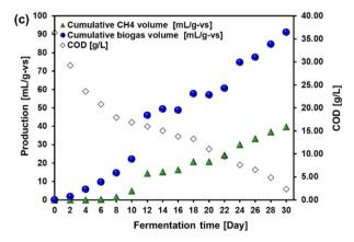
Fig. 4 Effect of algae-to-cow manure ratio on cumulative methane and biogas volume during the acclimatization process: algae-to-cow manure ratios of (a) 1:1, (b) 2:1, and (c) 3:1.
