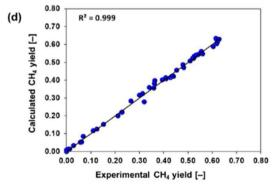
Fig. 7 Parity plots comparing the experimental data with the kinetic model using (a) first-order, (b) ternsference, (c) logistic, and (d) modified Gompertz model.
