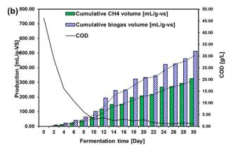
Fig. 5 (a) Gas composition after the acclimatization process and (b) cumulative methane and biogas volumes during anaerobic digestion following the acclimatization process using an algae-to-cow manure ratio of 2:1.
