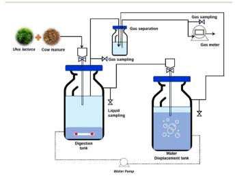
Fig. 1 A schematic representation of the reactor used for the biogas production from co-digestion of *U. lactuca* and cow manure.
