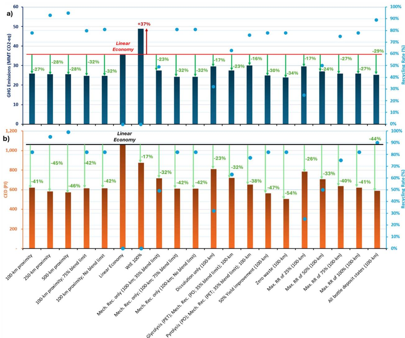
Fig. 9 Summary of optimal GHG emissions (primary Y-axis; in panel (a)) and CED impacts (primary Y-axis; in panel (b)) along with the respective recycling rates (secondary Y-axis) for all the scenarios modeled. Note: the dashed line represents the impacts of the linear economy scenario (80% landfill; 20% WtE) that serves as a basis for comparison. The percents of GHG emissions and CED savings relative to the linear economy scenario are shown in (a and b), respectively.
