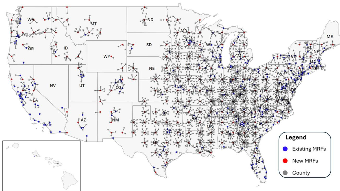
Fig. 3 County-to-MRF (C-2-M) optimal U.S. EOL PET and PO packaging recycling material flow network for systems optimized on GHG emissions with 100 km MRF collection proximity. Notes: (1) only the counties participating in recycling are shown in this figure; (2) Alaska has a 0% recycling rate, and therefore, is not shown in this figure. (3) This figure shows material flows from counties (origin) to MRFs (destination).
