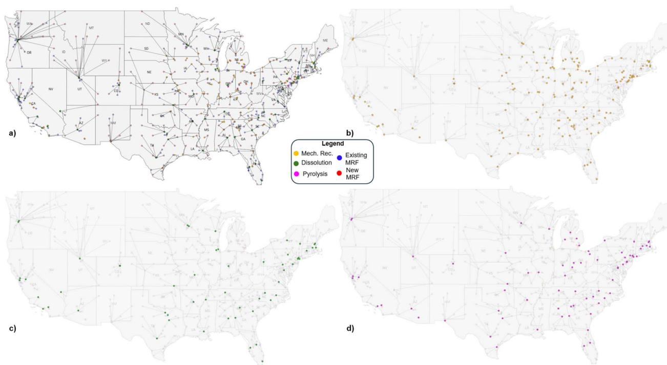
**Fig. 5** MRFs-to-PRFs (M-2-P) optimal U.S. EOL PET and PO packaging recycling material flow network for systems optimized on GHG emissions with 100 km MRF collection proximity. Notes: (1) this figure shows material flows from MRFs (origin) to PRFs (destination). (2) M-2-P material flows from Hawaii are shown in Fig. S21; † (3) the maps shown in (b–d) are slightly faded out to clearly highlight the locations of each recycling technology collectively shown in (a).
