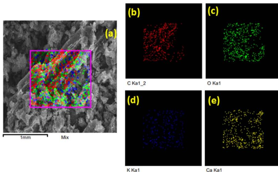
Fig. 6 Elemental mapping of (a) ALB displaying all the elements, (b) mapping of carbon, (c) mapping of oxygen, (d) mapping of potassium, and (e) mapping of calcium.
