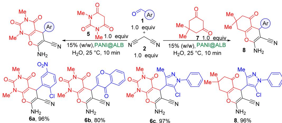
Scheme 3 Synthesis of pyrimidine-fused tetrahydropyrans and tetrahydro-4H-chromenes<sup>a</sup>. <sup>a</sup>Yields given were isolated after recrystallization in petroleum ether and ethanol. E-factor (0.04–0.25). E-factor = (mass of waste)/mass of the final product.
