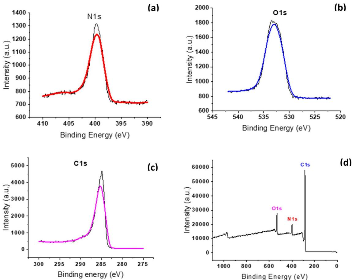
Fig. 11 High-resolution XPS spectrum of (a) N 1s, (b) O 1s, and (c) C 1s, and (d) XPS scan survey spectra of the PANI@ALB catalyst.
