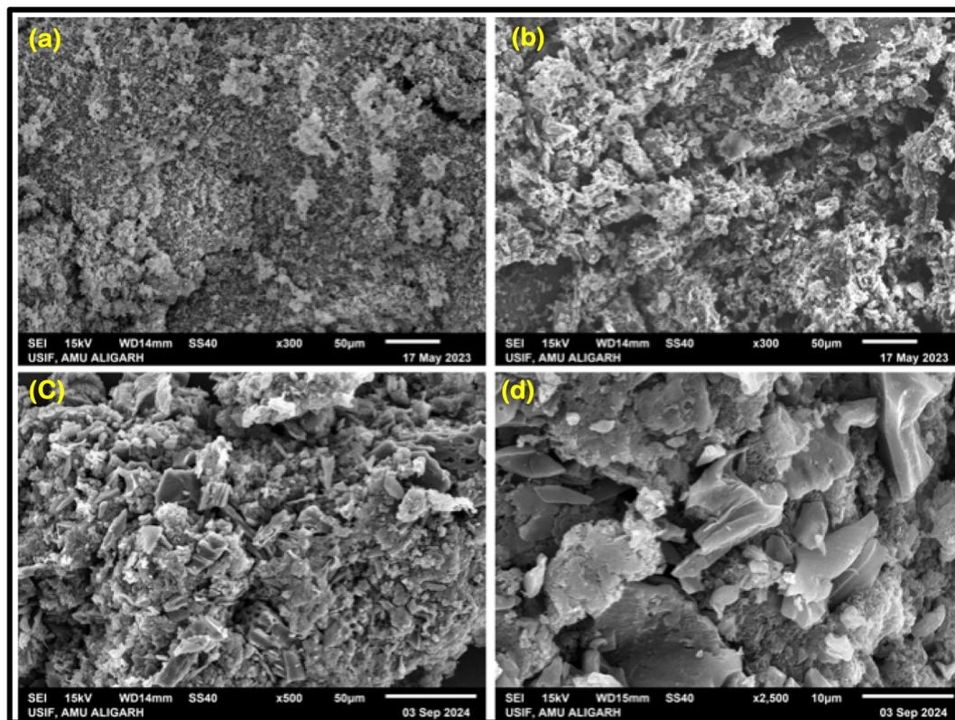
Fig. 3 SEM analysis of ALB (a and b) and PANI@ALB (c and d).
