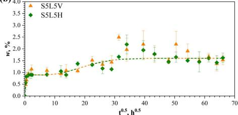
Fig. 6 Weight gain curves of vertically and horizontally printed specimens of (a) S5B5 and (b) S5L5. Lines are approximations by eqn (8)–(10).
