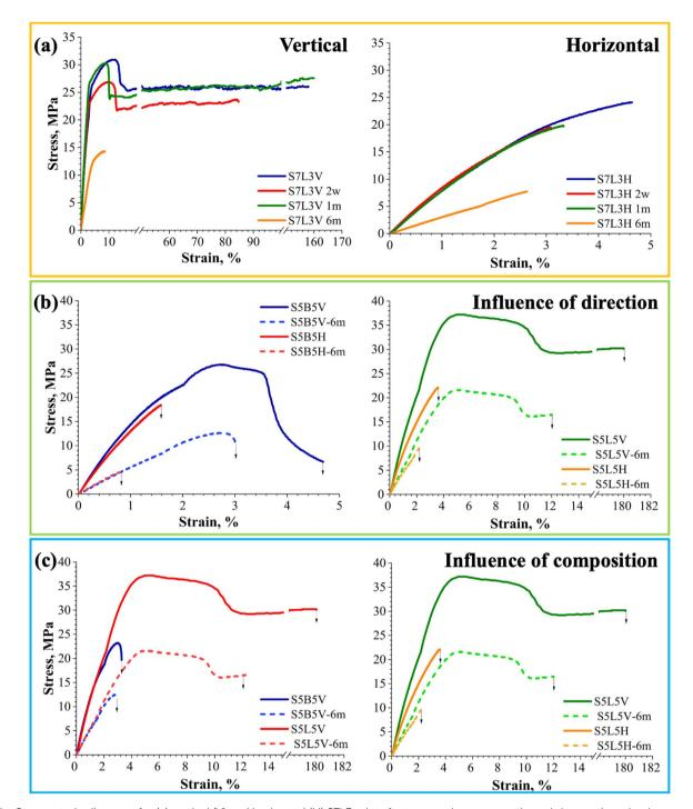
Fig. 10 Stress—strain diagrams for (a) vertical (V) and horizontal (H) S7L3 prints for two weeks, one month, and six months aging in seawater; (b) S5B5 and S5L5 vertical and horizontal prints; (c) S5B5, S5L5, and S7B3, S7L3 vertical samples in referenced and after aging in artificial seawater.
