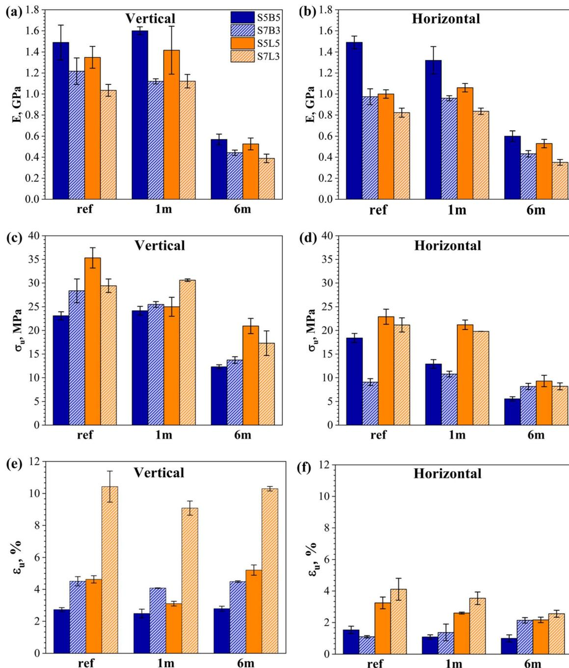
Fig. 11 (a) and (b) Elastic moduli ( $E$ ), (c) and (d) ultimate strength ( $\sigma_u$ ), (e) and (f) ultimate strain ( $\epsilon_u$ ) for PBS/PHB and PBS/PLA vertical and horizontal prints in the reference state and aged for one month and six months.
