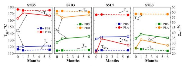
Fig. 9 Melting temperature (dashed lines) and degree of crystallinity (solid lines) extracted from first-run DSC heating scans for neat polymers and for PBS/PLA and PBS/PHB blends.
