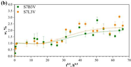
Fig. 5 Weight gain curves of vertically printed blend samples (a) S5B5 and S5L5, and (b) S7B3 and S7L3. Lines are approximations by eqn (8)–(10).
