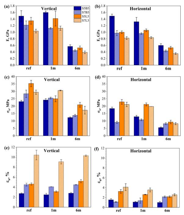
Fig. 11 (a) and (b) Elastic moduli (E), (c) and (d) ultimate strength (s<sub>11</sub>), (e) and (f) ultimate strain (e<sub>11</sub>) for PBS/PHB and PBS/PLA vertical and horizontal prints in the reference state and aged for one month and six months.
