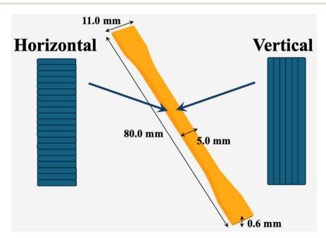
Fig. 1 Model of 3D printed dumbbell shape sample.
