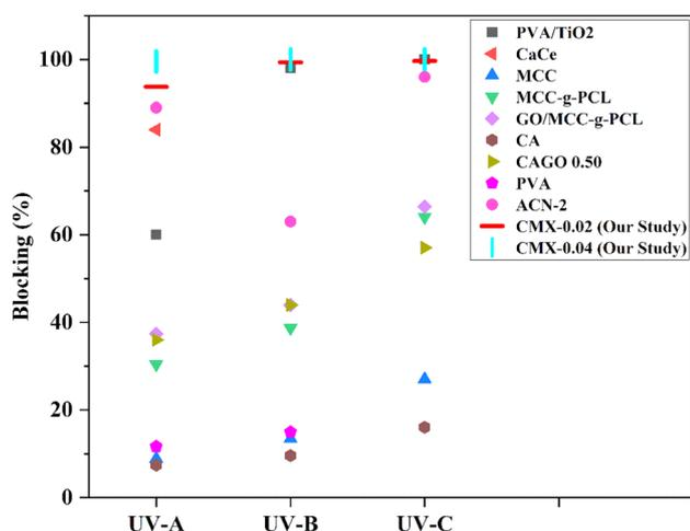
Fig. 8 UV radiation blocking performance of CMX nanocomposite films compared with other UV shielding materials available in the literature.<sup>12,70–76</sup>
