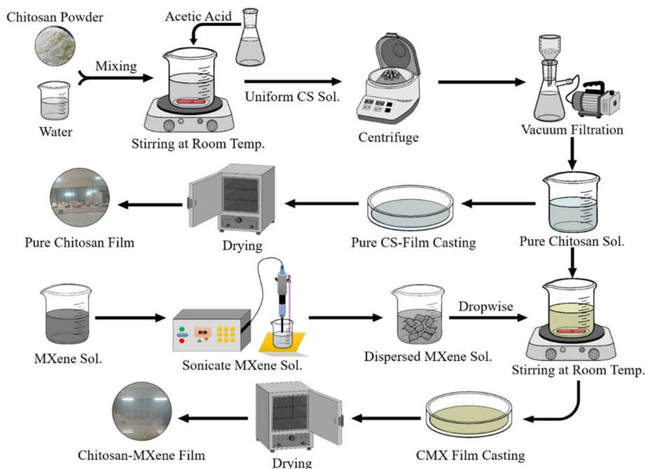
Fig. 2 Fabrication process of the UV-protective CMX film.
