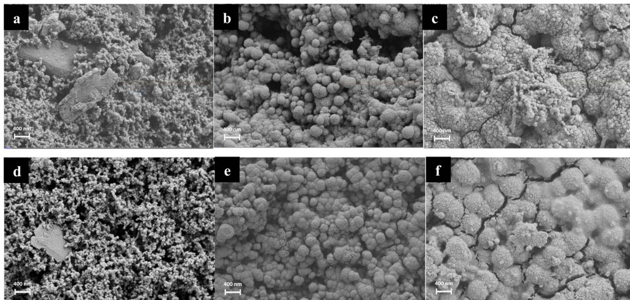
Fig. 6 Postmortem SEM images of BM-BH-SiO<sub>2</sub>/C and graphite anodes at different cycling stages under a C/5 current. (a–c) BM-BH-SiO<sub>2</sub>/C anode before cycling, after 10 cycles, and after 100 cycles, respectively. (d–f) Graphite anode before cycling, after 10 cycles, and after 100 cycles, respectively.
