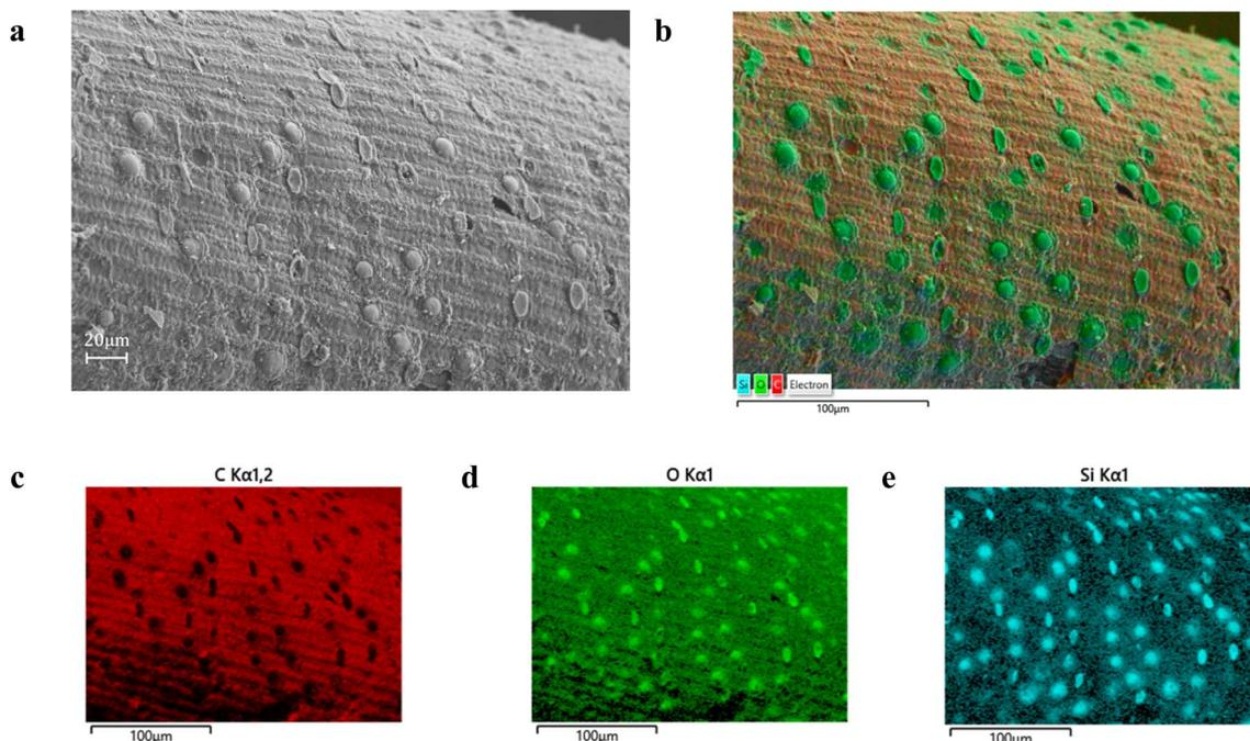
Fig. 1 (a) SEM image of BH-SiO<sub>2</sub>/C powder sample after acid wash, (b) corresponding EDX elemental mapping (Si, C, O), (c) carbon mapping, (d) oxygen mapping, and (e) silicon mapping.
