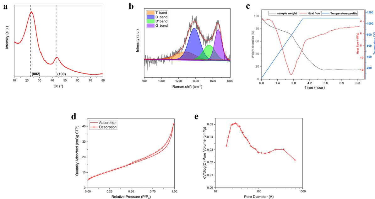
Fig. 3 (a) XRD pattern, (b) Raman spectra, (c) TGA/DSC, (d) nitrogen adsorption–desorption isotherms, and (e) pore size distribution of BM-BH-SiO<sub>2</sub>/C sample.
