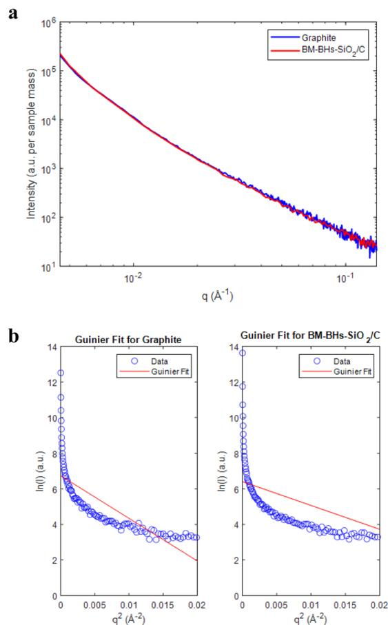
Fig. 4 (a) Log–log plot of scattering intensity  $I(q)$  vs. scattering vector  $q$ , and (b) Guinier fits showing  $\ln(I(q))$  vs.  $q^2$  for  $R_g$  determination for graphite and BM-BH-SiO<sub>2</sub>/C.
