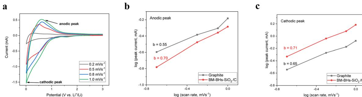
Fig. 7 (a) CV curves of the BM-BH-SiO<sub>2</sub>/C anode at varying scan rates (0.2, 0.5, 0.8, and 1.0 mV s<sup>-1</sup>), (b) log(*i*)–log(*v*) plot for anodic peak currents to determine the *b*-value, and (c) log(*i*)–log(*v*) plot for cathodic peak currents to determine the *b*-value.
