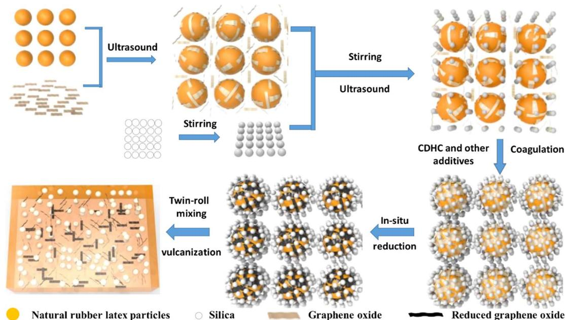
Fig. 5 Wet compounding procedure combined with an ultrasonic-assisted latex mixing route for preparing rGO/SiO<sub>2</sub>/NR nanocomposites. Reproduced with permission from ref. 46 Copyright (2020) MDPI.
