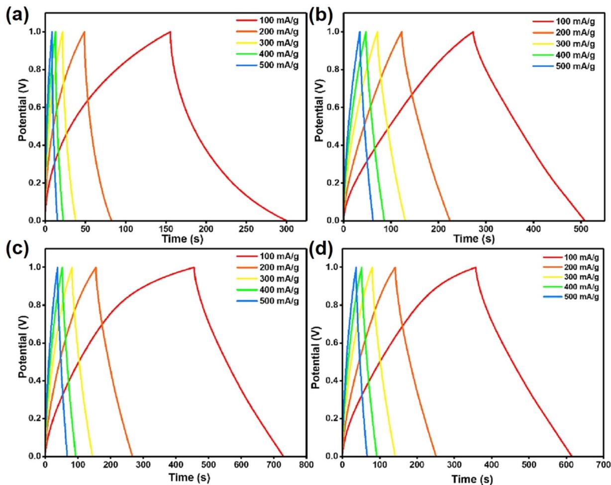
Fig. 12 GCD curves at different scan rates of symmetric EDLCs: (a) PC/S0/PC, (b) PC/S24/PC, (c) PC/S48/PC, and (d) PC/S72/PC. Reproduced with permission from ref. 47 Copyright (2023), Elsevier Inc.
