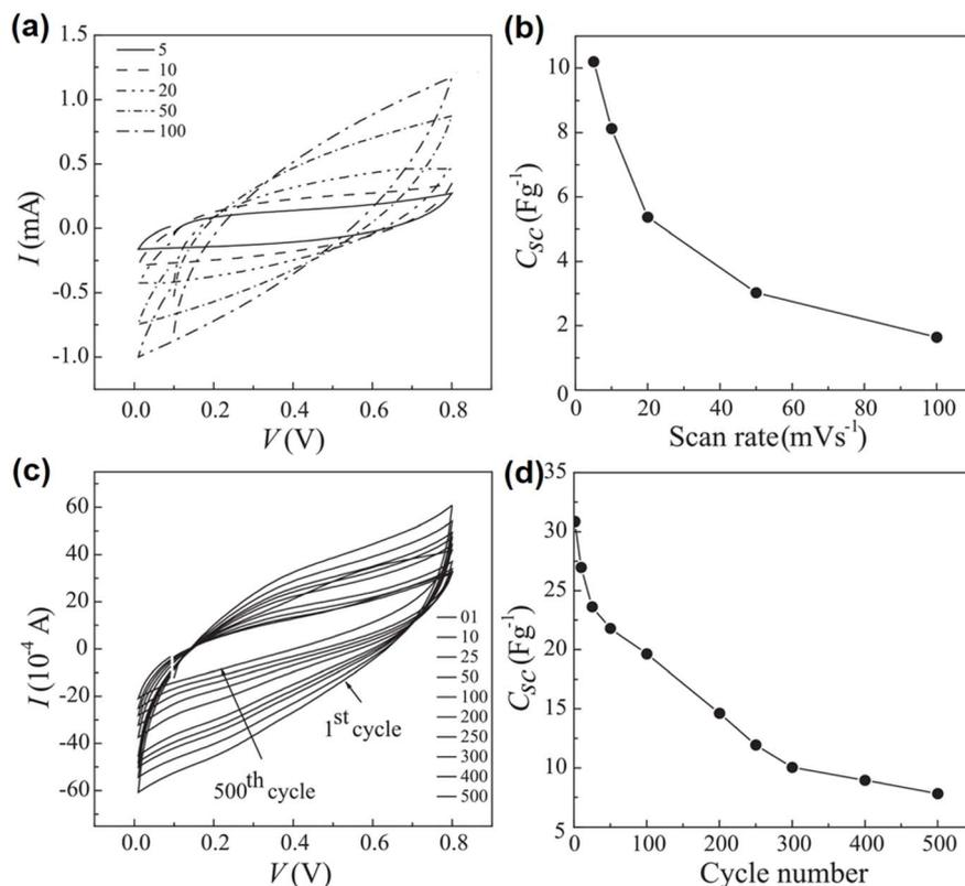
**Fig. 10** (a) CV curves at different scan rates; (b) capacitance variation with respect to scan rates; (c) CV curves at different cycle numbers (1 to 500); and (d) plot of variation in the specific capacitance of the single electrode for 500 continuous cycles at a fixed scan rate of 10  $\text{mV s}^{-1}$ . Reproduced with permission from ref. 63 Copyright (2023), Wiley-VCH Verlag VCH Ltd.
