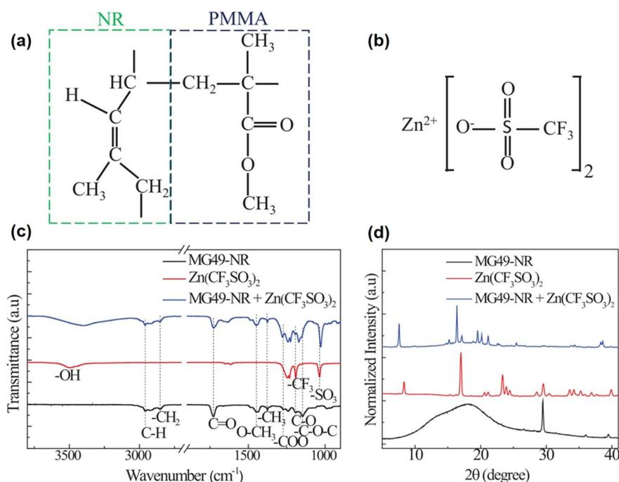
Fig. 9 Schematic of (a) MG<sub>49</sub>-NR and (b)  $\text{Zn}(\text{CF}_3\text{SO}_3)_2$  and (c) attenuated total reflectance FTIR and (d) XRD spectra of the proposed samples. Reproduced with permission from ref. 63 Copyright (2023), Wiley Verlag VCH.
