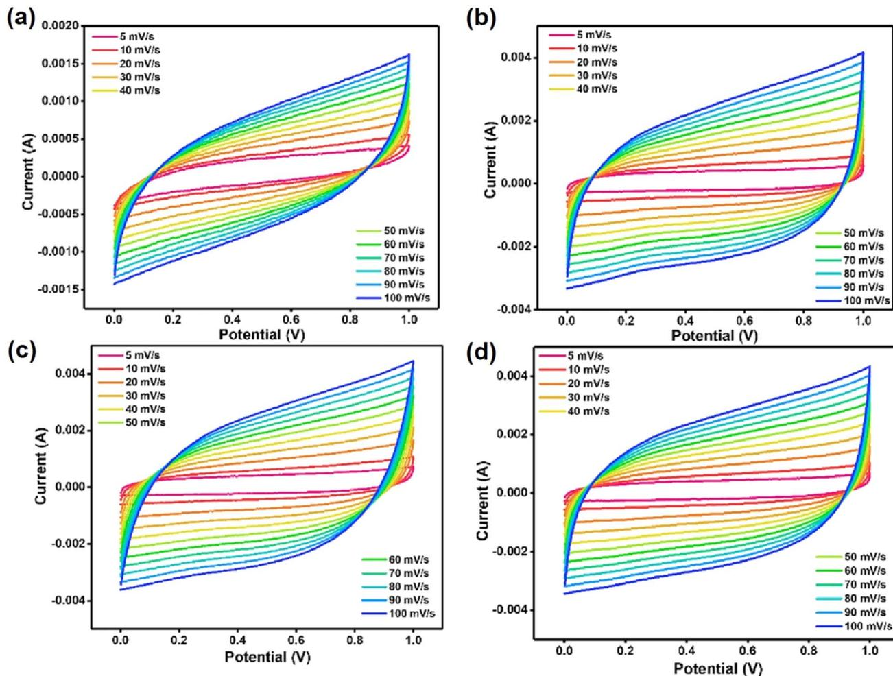
Fig. 11 CV curves at different scan rates of symmetric EDLCs: (a) PC/S0/PC, (b) PC/S24/PC, (c) PC/S48/PC, and (d) PC/S72/PC. Reproduced with permission from ref. 47 Copyright (2023), Elsevier Inc.
