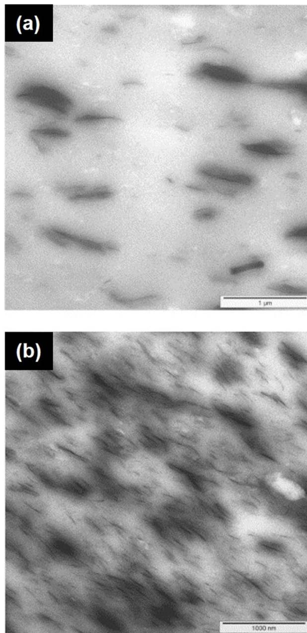
Fig. 4 TEM images of an (a) NR with DDA clay and (b) NR with ODA-modified clay. Reproduced with permission from ref. 52 Copyright (2005), Elsevier Inc.
