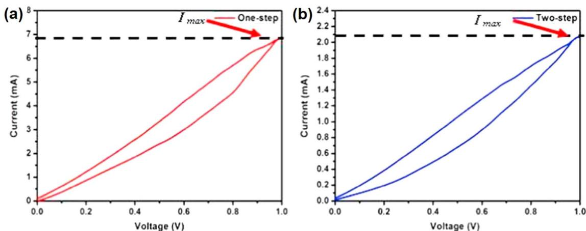
Fig. 7 CV profiles of the GO/NRL nanocomposite electrodes prepared *via* the (a) one-step mixing method and (b) two-step mixing method. Reproduced with permission from ref. 57 Copyright (2015), Elsevier Inc.
