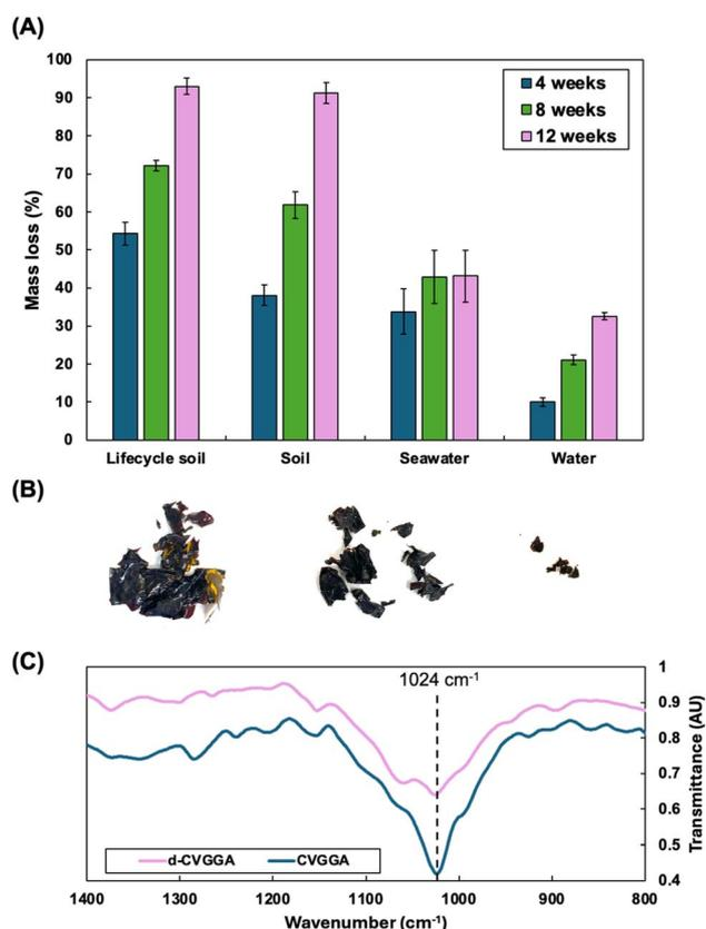
Fig. 6 (A) Degradation of CVGGA films in soil after submersion in food simulant (lifecycle), soil, seawater and water, (B) images of CVGGA films during degradation in soil, taken after rinsing with water and drying, (C) FTIR comparison of CVGGA and soil-degraded CVGGA films.
