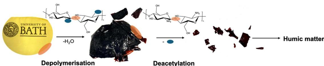
Fig. 8 Schematic of the proposed mechanism of degradation for CVGGA films, where the first stage involves depolymerisation via hydrolytic cleavage of glycosidic bonds, likely starting at the outside of the film, followed by deacetylation and cleavage of Schiff-base bonds, followed by further degradation and assimilation to humic matter.
