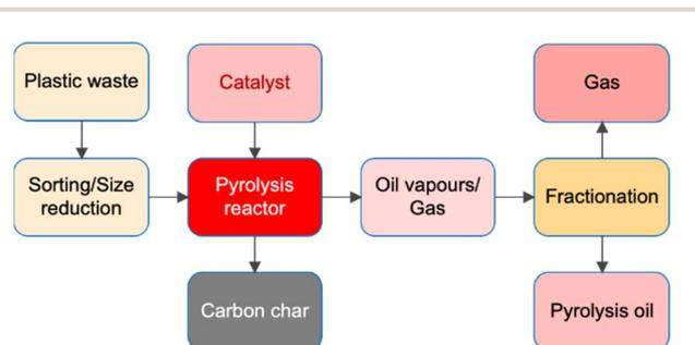
Fig. 10 Basic flow diagram of the pyrolysis process.
