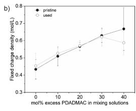
Fig. 3 (a) Water uptake of saloplastic membranes at different KCl concentrations, measured at 25 °C. (b) Fixed charge density of saloplastic membranes in both pristine form and after testing and long-term storage in 0.5 M KCl (used). Each point represents the mean of at least three measurements, with the 95% confidence interval indicated as the error margin. Lines are guides for the eye to highlight the general trend of the data
