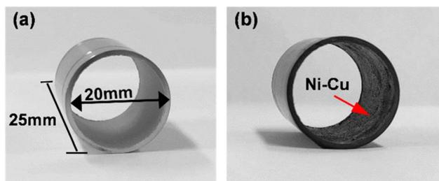
Fig. 1 Overview of the stainless-steel hollow-wall-type catalyst. (a) Before and (b) after electroless plating.
