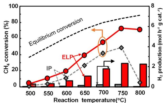
Fig. 10 Comparing the H<sub>2</sub> production and CH<sub>4</sub> conversion of the ELP- and IP-derived catalysts.
