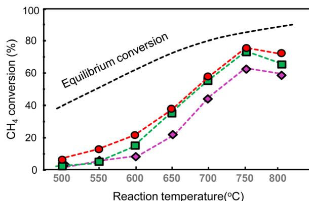
Fig. 8 Effect of reduction temperature on the methane-decomposition performance of the 70–30 Ni–Cu catalyst.
