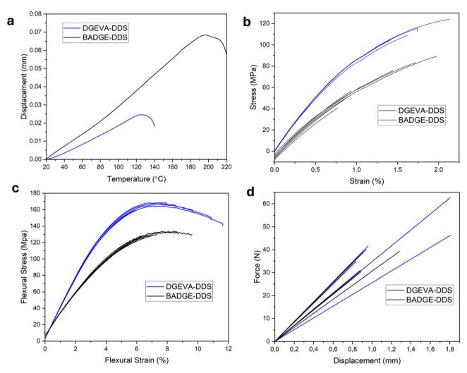
Fig. 4 (a) TMA displacement vs. temperature graphs for both systems. (b) Tensile stress-strain curves. (c) Flexural stress-strain curves. (d) Fracture toughness force-displacement graph. BADGE-DDS results from a previous study published by our group.<sup>7</sup>
