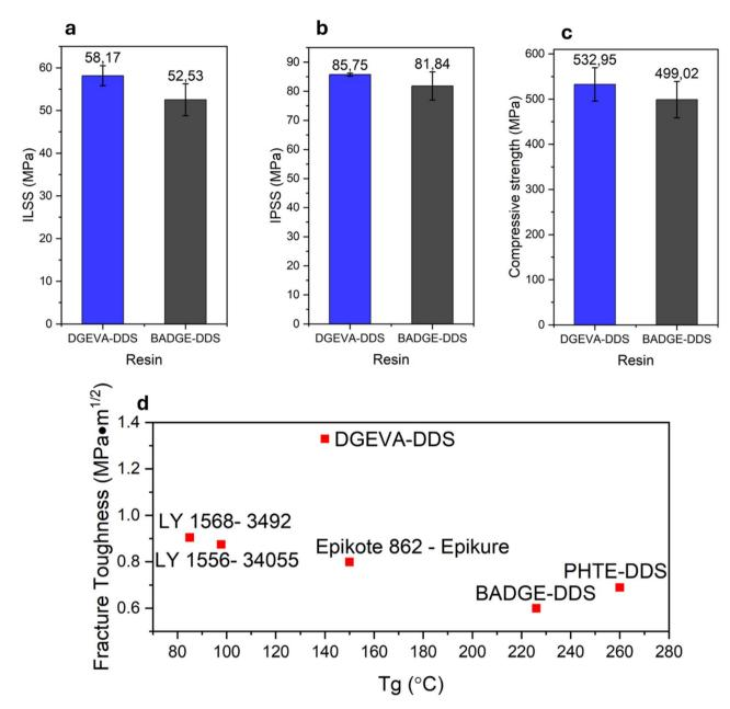
Fig. 6 (a) ILSS results. (b) IPSS results. (c) Compression strength results. (d) Fracture toughness vs.  $T_q$  for a variety of epoxy-amine systems.
