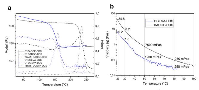
Fig. 2 (a) DMA temperature sweep in the three point bending setup of both systems. Heating rate  $= 1 \text{ K min}^{-1}$ . (b) Viscosity vs. temperature profiles of both systems.
