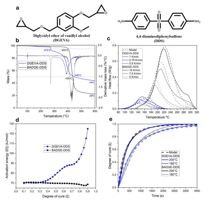
Fig. 1 (a) Chemical structures of DGEVA epoxy and DDS hardener. (b) TGA of cured resins. (c) Isothermal DSC thermograms and corresponding modelling fits. (d)  $E_a$  evolution vs. degree of cure for both resin systems. (e) Degree of cure vs. time at isothermal temperatures.
