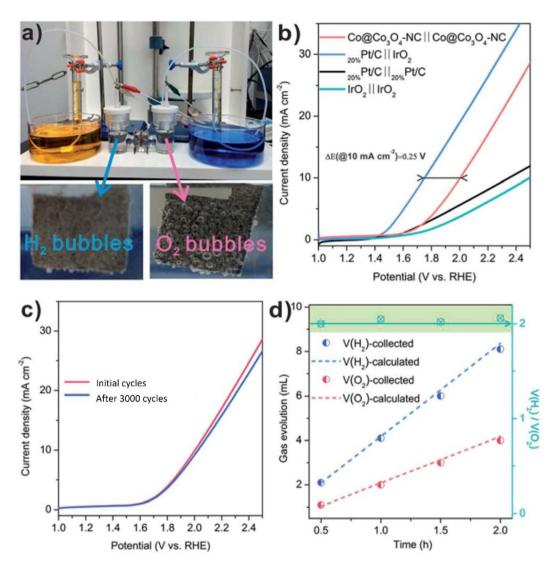
Fig. 7 (a) Photograph of the two-electrode water splitting and gas collection device. (b) Polarization curves of  $Co@Co_3O_4$ -NC|| $Co@Co_3O_4$ -NC, Pt/C||| $IrO_2$ , Pt/C|||| $IrO_2$ , Pt/C|||| $IrO_2$ , Pt/C||||
