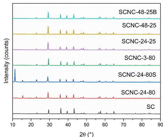
Fig. 5 X-ray diffractograms of soft calcite/copper oxide NCs and the control sample (bottom to top: black, soft calcite (SC) unmodified as the control sample; red, SCNC-24-80; blue, SCNC-24-80S; green, SCNC-3-80; purple, SCNC-24-25; yellow, SCNC-48-25; aqua, SCNC-48-25B).
