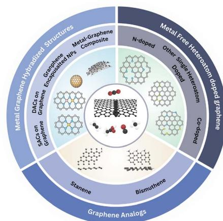
Fig. 1 Schematic representation categorizing graphene-based catalysts designed for eCO<sub>2</sub>RR.
