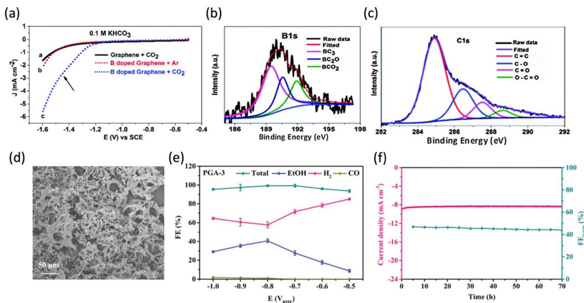
Fig. 9 Other heteroatom doped graphene for eCO<sub>2</sub>RR High-resolution XPS spectra of (a) B1s and (b) C1s (c) LSV of BG and Bi in 0.1 M KHCO<sub>3</sub> in the presence of CO<sub>2</sub>. Adapted with permission from ref. 85 Copyright 2015, Royal Society of Chemistry. (d) SEM image of PGA-2. (e) Stability test on PGA-2. (f) FE for EtOH and yield for PGA-2 in a flow cell. Adapted with permission from ref. 19 Copyright 2022, Wiley.
