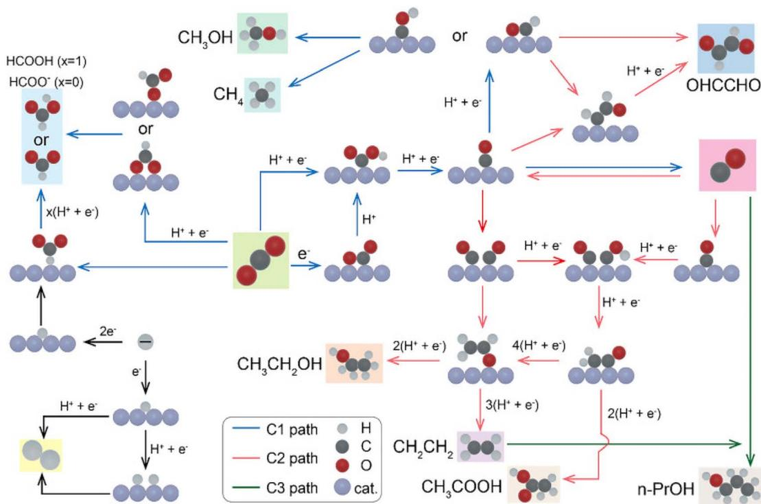
Fig. 2 Mechanistic pathways for electrochemical CO<sub>2</sub> reduction to C<sub>1</sub>, C<sub>2</sub>, and C<sub>3</sub> products. Adapted with permission from ref. 22 Copyright 2023, Elsevier.
