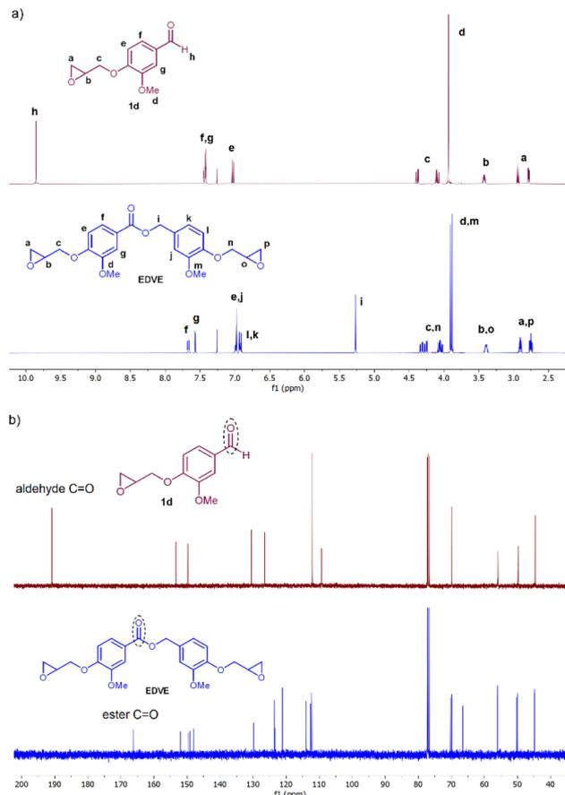
Fig. 3 (a)  $^1\text{H}$  NMR spectrum of vanillin epoxide **1d** (top) and EDVE (bottom) in  $\text{CDCl}_3$ ; (b)  $^{13}\text{C}$  NMR spectra of vanillin epoxide **1d** (top) and EDVE (bottom) in  $\text{CDCl}_3$ .
