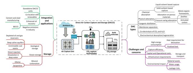
Fig. 7 Conceptual overview of direct air carbon capture and storage (DACCS) systems, including core technologies, storage options, DAC types, integration opportunities, and key challenges.
