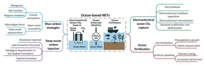
Fig. 12 Overview of ocean-based NETs, including blue carbon strategies, deep ocean carbon injection, electrochemical ocean CO<sub>2</sub> capture, ocean enhanced alkalinity, and ocean fertilization.
