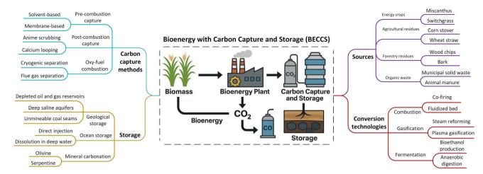
Fig. 5 Conceptual layout of bioenergy with carbon capture and storage (BECCS), illustrating sources, conversion technologies, carbon capture processes, and CO<sub>2</sub> transport and storage pathways.
