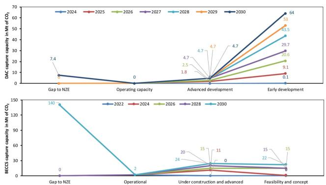
Fig. 6 CO<sub>2</sub> capture capacity comparison of planned BECCS and DACCS projects (2022-2030) (data from ref. 92).
