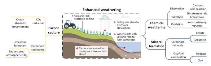
Fig. 10 Process of enhanced weathering for carbon capture and storage through chemical weathering and mineral formation (conceptual layout adapted from ref. 128)
