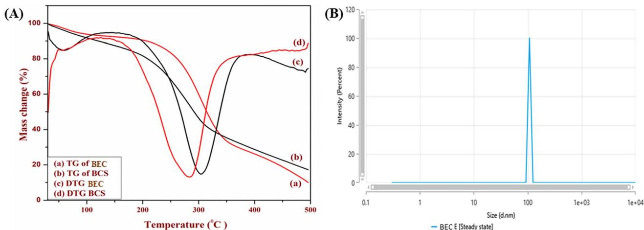
Fig. 4 (A) Thermal analysis of BEC and BCS and (B) DLS of BEC.
