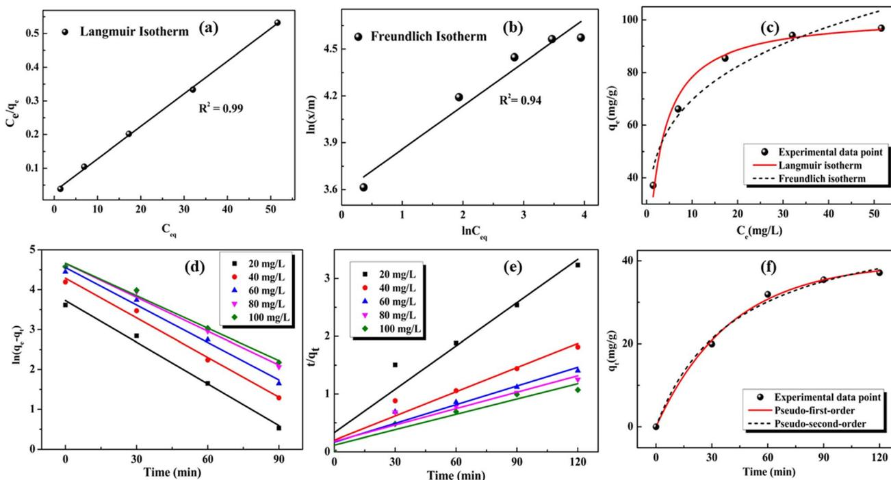
Fig. 8 At pH = 6 and an adsorbent amount of  $0.5 \text{ g L}^{-1}$ , the graph of (a) Langmuir and (b) Freundlich adsorption isotherms of MG. (c) Nonlinear fitting plots for both adsorption isotherms (d) pseudo-first-order kinetics, (e) pseudo-second-order kinetics of MG dye and (f) non-linear fitting plot for the kinetics of adsorption (temp. =  $25^\circ \text{C}$ ) for 20 mg per L MG dye solution.
