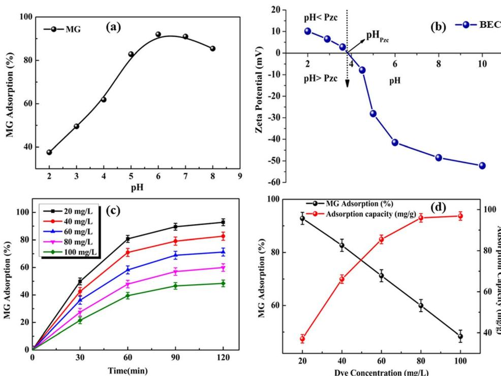
Fig. 7 (a) Effect of pH (adsorbent amount =  $0.5 \text{ g L}^{-1}$ ; MG dye conc. =  $20 \text{ mg L}^{-1}$ ; temperature =  $25 \text{ }^{\circ}\text{C}$ ), (b)  $\text{pH}_{\text{PZC}}$  of the BEC adsorbent, (c) effect of adsorption time, and (d) effect of dye concentration on MG dye removal by the BEC adsorbent ( $\text{pH} = 6$ ; adsorbent amount =  $0.5 \text{ g L}^{-1}$ ; contact time = 120 min; temp. =  $25 \text{ }^{\circ}\text{C}$ ).
