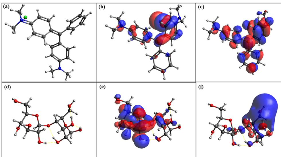
Fig. 3 Optimized molecular structure of (a) malachite green, and its (b) HOMO and (c) LUMO and (d) the optimized molecular structure of cellobiose, and its (e) HOMO and (f) LUMO.
