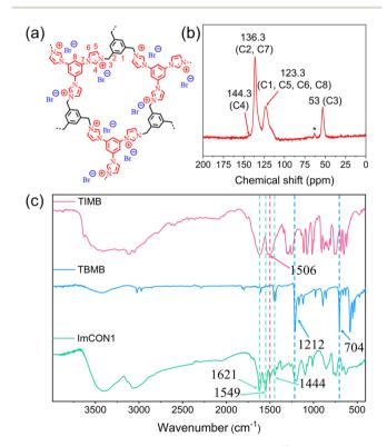
Fig. 1 (a) Structure of ImCON1, (b) solid-state <sup>13</sup>C CP-MAS NMR spectrum of ImCON1 (the peak marked with \* is the spinning sideband), (c) FTIR spectrum of ImCON1 compared with monomers.
