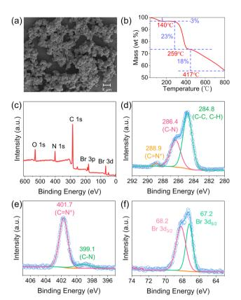
Fig. 2 (a) SEM image, (b) TGA curve, and XPS spectra of ImCON1 (c) survey, (d) C 1s, (e) N 1s and (f) Br 3d.
