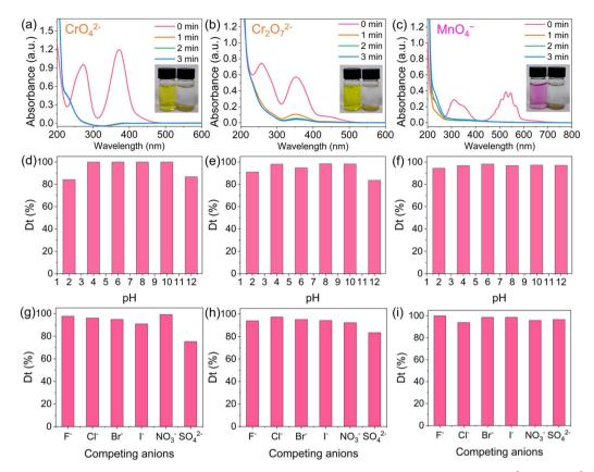
Fig. 3 UV-vis spectroscopy in the presence of ImCON1 at different time intervals for the water solution of (a)  $CrO_4^{2-}$ , (b)  $Cr_2O_7^{2-}$  and (c)  $MnO_4^{-}$ ; effect of pH value on the capture efficiency of (d)  $CrO_4^{2-}$ , (e)  $Cr_2O_7^{2-}$  and (f)  $MnO_4^{-}$  by ImCON1; the bar diagrams represent the removal efficiency of ImCON1 in the presence of competing anions for (g)  $CrO_4^{2-}$ , (h)  $Cr_2O_7^{2-}$  and (i)  $MnO_4^{-}$ .
