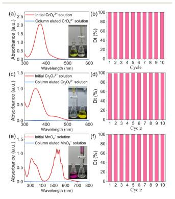
Fig. 4 Column adsorption experiments: UV-vis spectra for the solution of (a)  ${\rm CrO_4}^{2-}$ , (c)  ${\rm Cr_2O_7}^{2-}$  and (e)  ${\rm MnO_4}^-$  before and after passage through the column (inset: photograph of the column adsorption experiment for oxo-anion capture). Recyclability of ImCON1 for adsorption of (b)  ${\rm CrO_4}^{2-}$ , (d)  ${\rm Cr_2O_7}^{2-}$  and (f)  ${\rm MnO_4}^-$ .
