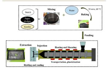
Fig. 1 Scheme of injection moulding process from the dough kneading (upper picture) to the tray extraction (lower picture) after compression moulding at 155 °C.
