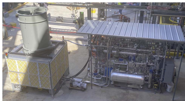
Fig. 5 One of Aircapture's DAC units (left) and collection skid (right). Located in Wilsonville, Alabama, USA at the US National Carbon Capture Center, this unit has been operating since March 2023.
