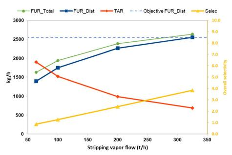
Fig. 3 Furfural and tars production and the overall selectivity among them (kg of furfural distilled per kg of tars) in function of the stripping vapor flow (200 °C). "FUR\_total" accounts for the total furfural output (distillated + waste stream) in the reactor. "FUR\_Dist" is the flow of furfural that leaves the reactor with the stripping steam. "Objective FUR\_Dist" accounts for the furfural flow that leaves the reactor with the stripping steam in CBP.
