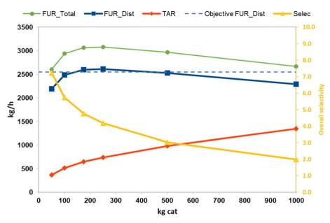
Fig. 5 Effect of the catalyst amount on the furfural and tars production and their selectivity at 200 °C and using 25 kg of stripping vapor per kg furfural. "FUR\_total" accounts for the total furfural output (distilled + waste stream) in the reactor. "FUR\_Dist" is the flow of furfural that leaves the reactor with the stripping steam. "Objective FUR\_Dist" accounts for the furfural flow that leaves the reactor with the stripping steam in CBP.
