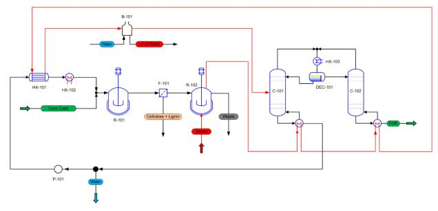
Flowsheet diagram of HCP (red lines indicate the stripping steam streams carrying furfural from the reactor to the first distillation column).
