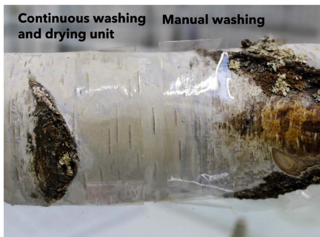
Fig. 4 Photograph of the films washed and dried by the use of the continuous unit (left) and manually (right) over a wood log.
