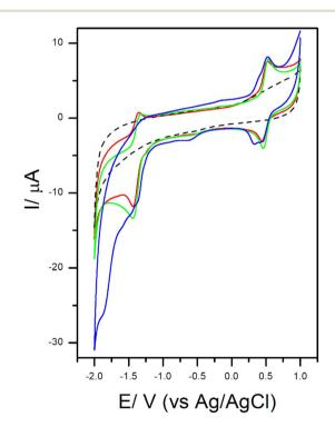
Fig. 1 Electrochemical behavior of BMImBF<sub>4</sub> used as solvent (dashed black line), a solution containing 9 mM of Ni(cyclam)Cl<sub>2</sub> and N<sub>2(sat)</sub> (red), addition of propylene oxide (10 mM) saturated with N<sub>2</sub> (green) and saturated with  $CO_2$  (blue). Scan rate: 100 mV s $^{-1}$ , WE: glassy carbon, CE: Pt coil and RE: Ag/AgCl(sat)
