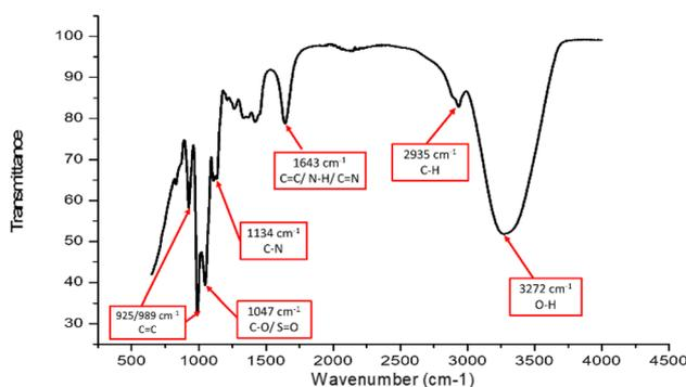
Fig. 13 FTIR spectrum of the optimized CQDs.
