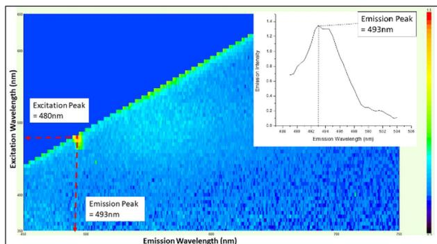
Fig. 3 3-D measurement of the excitation wavelength and the emission wavelength for CQDs produced via the microwave irradiation method. Inset shows the corresponding emission spectrum.
