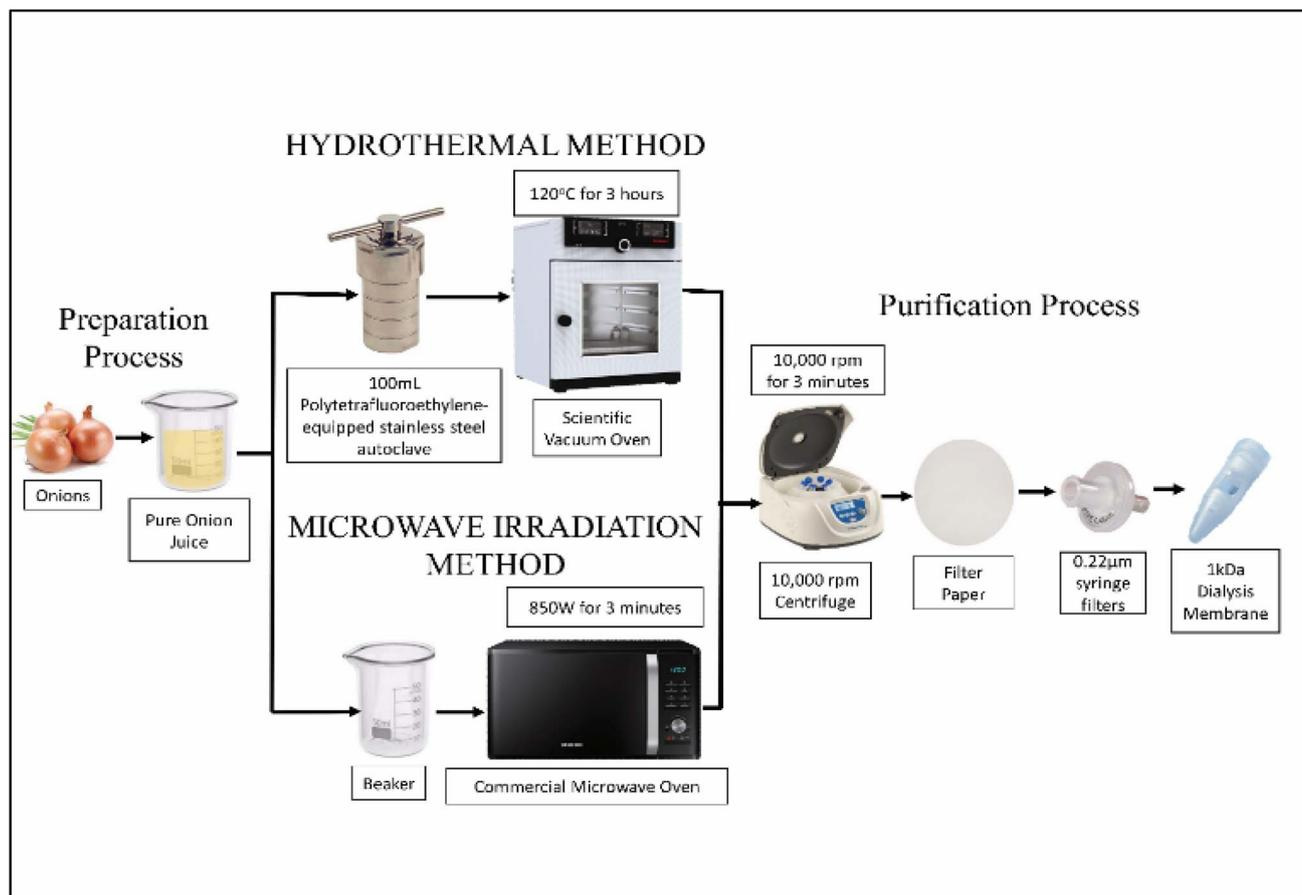
Fig. 1 Preparation, synthesis, and purification of CQDs.
