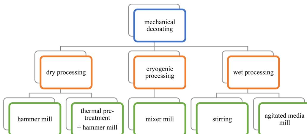
Fig. 2 Experiments (green) carried out on the different approaches (orange) for mechanical decoating.
