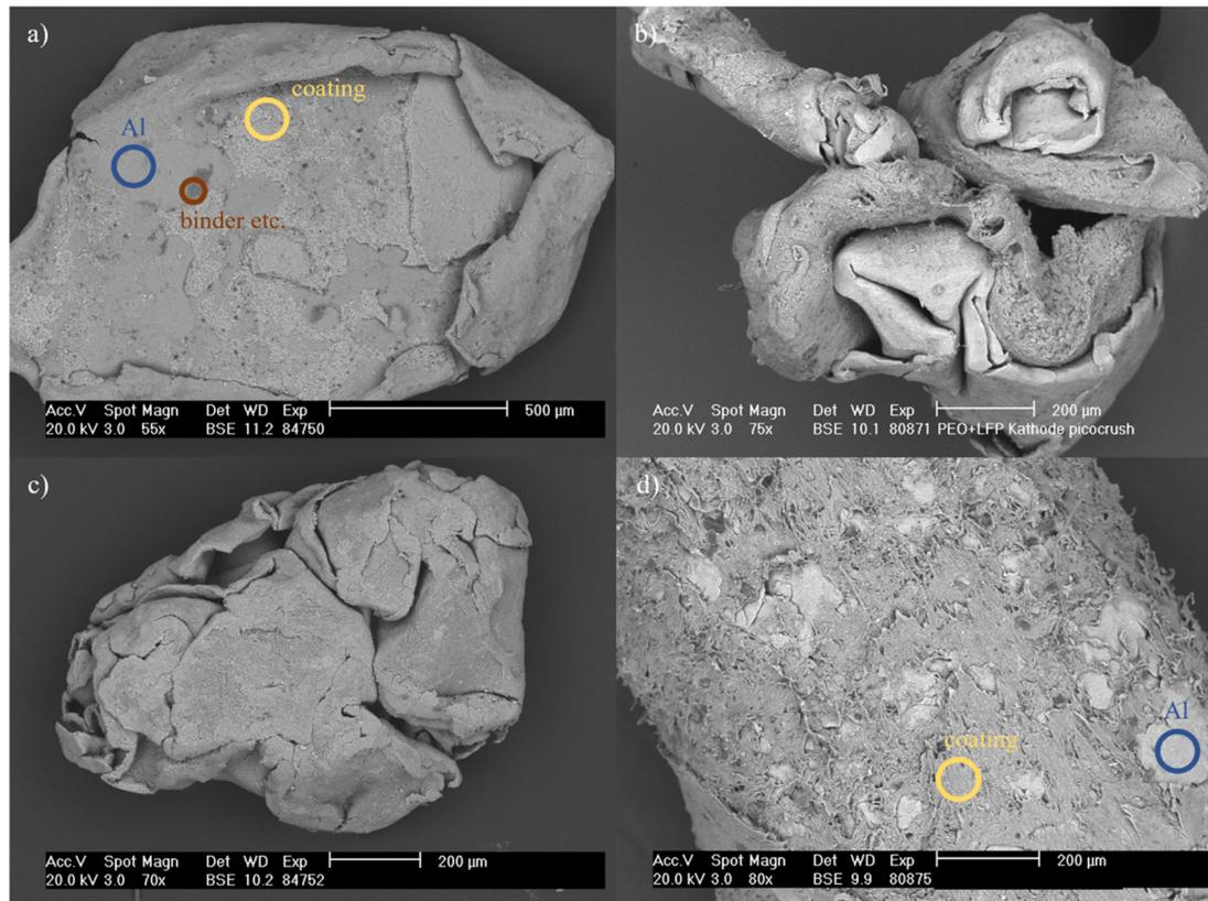
Fig. 4 Cathode sheet particles after mechanical stressing in the hammer mill at 25 m s<sup>-1</sup> with (a) conventional LFP cathode, (b) PEO/LFP cathode, (c) PEO/LFP cathode with prior thermal treatment and (d) PEO/LFP cathode after cryogenic comminution.
