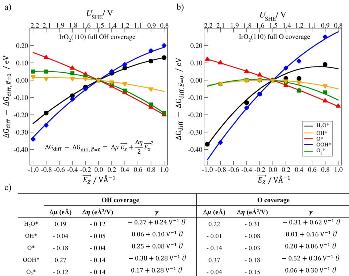
Fig. 3 Field response of the relevant intermediates in OER on IrO<sub>2</sub>(110) under (a) OH\* coverage and (b) O\* coverage on Ir<sub>CUS</sub> sites. (c) Table with fitted values for the change in surface dipole ( $\Delta\mu$ , [eÅ]) and polarizability ( $\Delta\eta$ , [ $\frac{\text{e}\text{\AA}^2}{\text{V}}$ ]) associated with a change in surface phase. Additionally, the net potential response for each adsorbate is indicated where  $\bar{U} = U_{\text{SHE}} - U_{\text{PZC}}$ .
