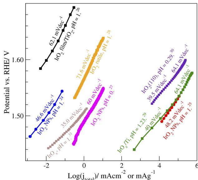
Fig. 1 Experimental Tafel plots for OER on IrO<sub>x</sub>-based catalysts in acidic conditions. Square and circle symbols represent films and nanoparticles (NPs), respectively.<sup>24–31</sup> Note that the reported current densities ( $j_{\text{total}}$ ) vary in their normalization, making the direct comparison of  $j_{\text{total}}$  unjustified. This does not affect the highlighted Tafel slope values.
