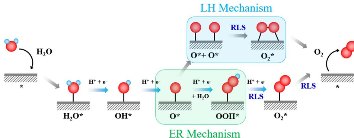
**Scheme 1** Schematic illustration of the possible reaction mechanism for OER on IrO<sub>2</sub>(110). The O<sub>2</sub> molecule is formed by O–O bond formation either by a Langmuir–Hinshelwood (LH) mechanism or Eley–Rideal (ER) mechanism *via* a coupled proton–electron transfer. Possible rate-limiting steps (RLS) are marked in blue and green colors.
