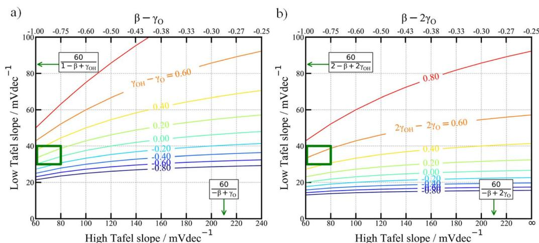
Fig. 2 Tafel slopes considering (a) the ER mechanism (O–OH formation) and (b) the LH mechanism (O–O coupling). Contours show the variation in the Tafel slope considering the potential response ( $\gamma$ ) of OH\* and O\* for estimating low (y-axis) and high (x-axis) Tafel slopes, respectively. Experimentally observed Tafel slopes are marked with a dark green box.
