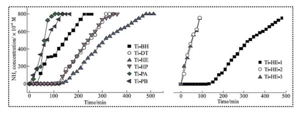
Fig. 13 NH $_3$  adsorption efficiency of PTPs (left) and three cycles of NH $_3$  adsorption measurements for Ti-HE. Adapted with permission from ref. 60. Copyright of Wuhan University of Technology and Springer Verlag Berlin Heidelberg, 2017.
