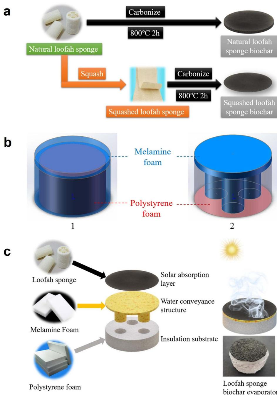
**Fig. 11** (a) Synthesis process of loofah sponge biochar solar absorption layer. (b) Schematic representation of structure of internal and external water conveyance substrate. (c) Schematic comparison of structure of a loofah sponge biochar evaporator. Reproduced with permission from ref. 42. Copyright (2022) Elsevier Inc.
