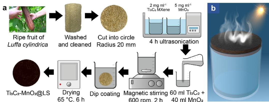
Fig. 17 (a) Schematic representation of the synthesis process of  $\text{Ti}_3\text{C}_2$ - $\text{MnO}_2$ -loofah sponge hybrid. (b) Illustration showing the generation of solar steam using the  $\text{Ti}_3\text{C}_2$ - $\text{MnO}_2$ -loofah sponge hybrid. Reproduced with permission from ref. 70. Copyright (2023) Elsevier Inc.
