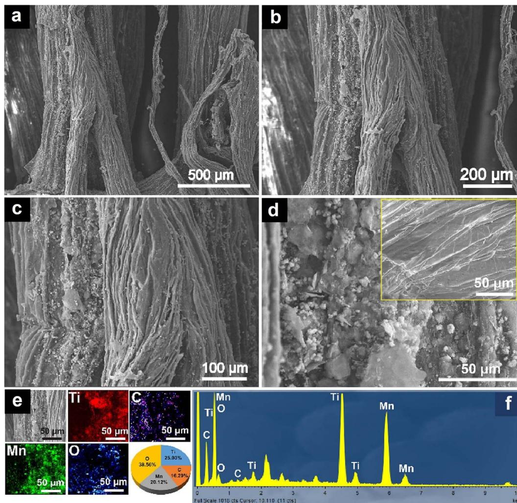
Fig. 18 (a–d) SEM images of Ti<sub>3</sub>C<sub>2</sub>-MnO<sub>2</sub>-coated loofah sponge with various magnifications. Inset of (d) shows pristine loofah sponge. (e) EDS elemental mapping. (f) EDS spectrum showing elemental analysis. Reproduced with permission from ref. 70. Copyright (2023) Elsevier Inc.
