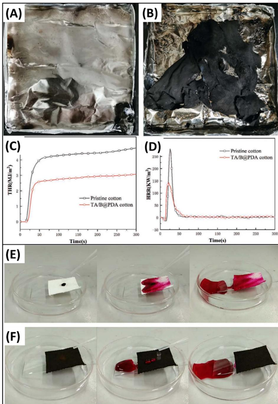
Fig. 6 Digital photographs of char residues of (A) pristine cotton and (B) TA/B@PDA cotton fabrics after CCT. (C) THR and (D) HRR of cotton samples, reproduced with permission from ref. 74; illustrations of fabric with reactive red dye powder under rinsing with water: (E) original cotton fabric and (F) Fe/PDA/ODA cotton fabric, reproduced with permission from ref. 5.
