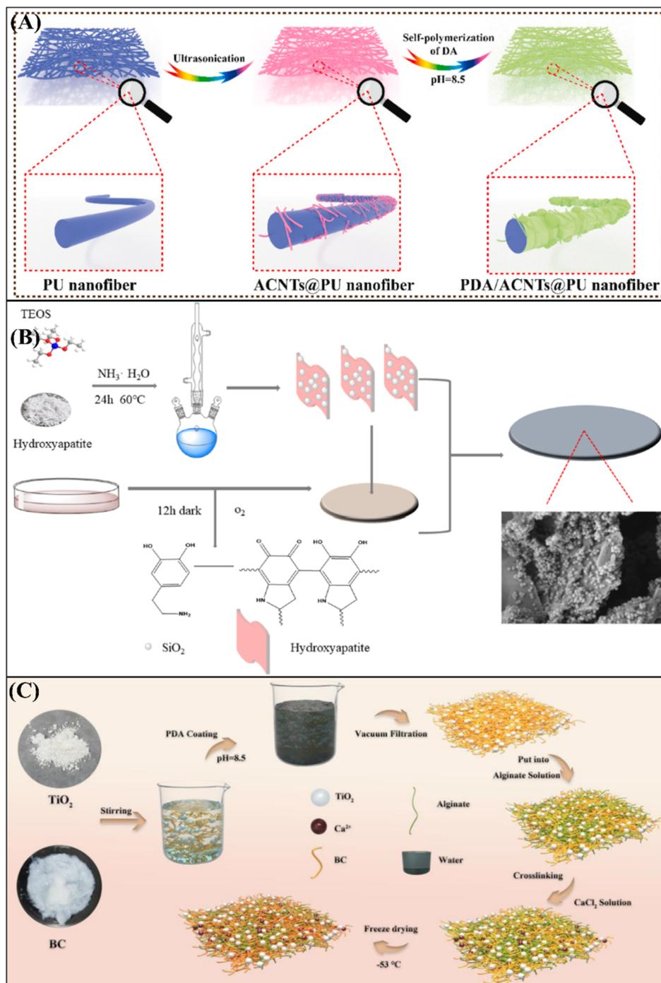
Fig. 14 Schematic illustration for preparation of composite membranes: (A) PDA@PU/ACNTs, reproduced with permission from ref. 122. (B) HAP/SiO<sub>2</sub>/PDA, reproduced with permission from ref. 100. (C) Bacterial cellulose/PDA/TiO<sub>2</sub>, reproduced with permission from ref. 101.
