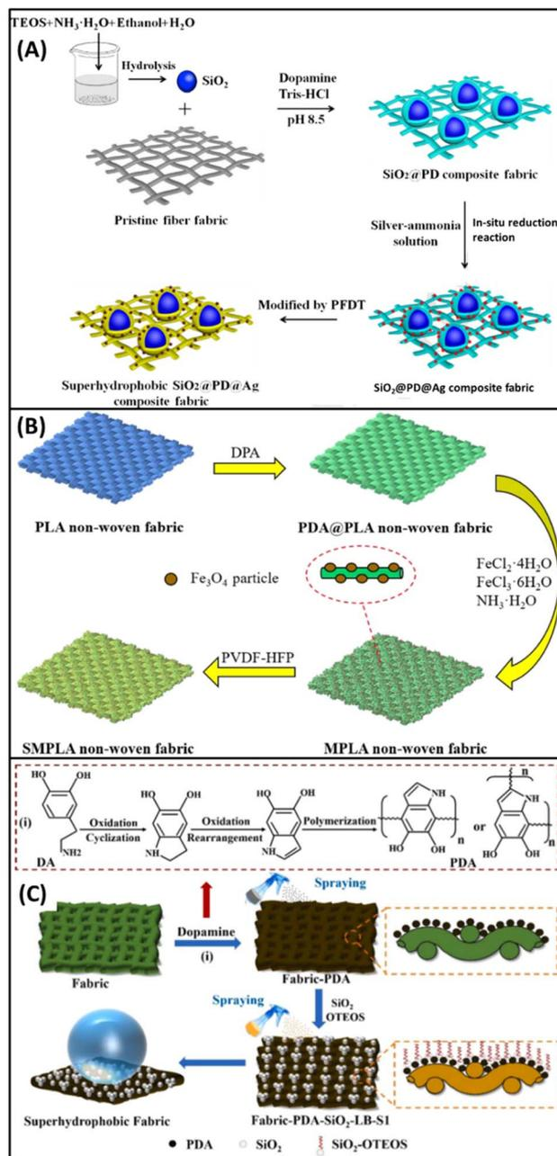
Fig. 9 Schematic illustration for the preparation of superhydrophobic fabrics (other than cotton): (A) tetra-copolyester and polypropylene/SiO<sub>2</sub>/PD/Ag/PFDT, reproduced with permission from ref. 75; PLA/PDA/PVDF-HFP (B), reproduced with permission from ref. 77; other materials/PDA/SiO<sub>2</sub>/OTEOS (C), reproduced with permission from ref. 82.
