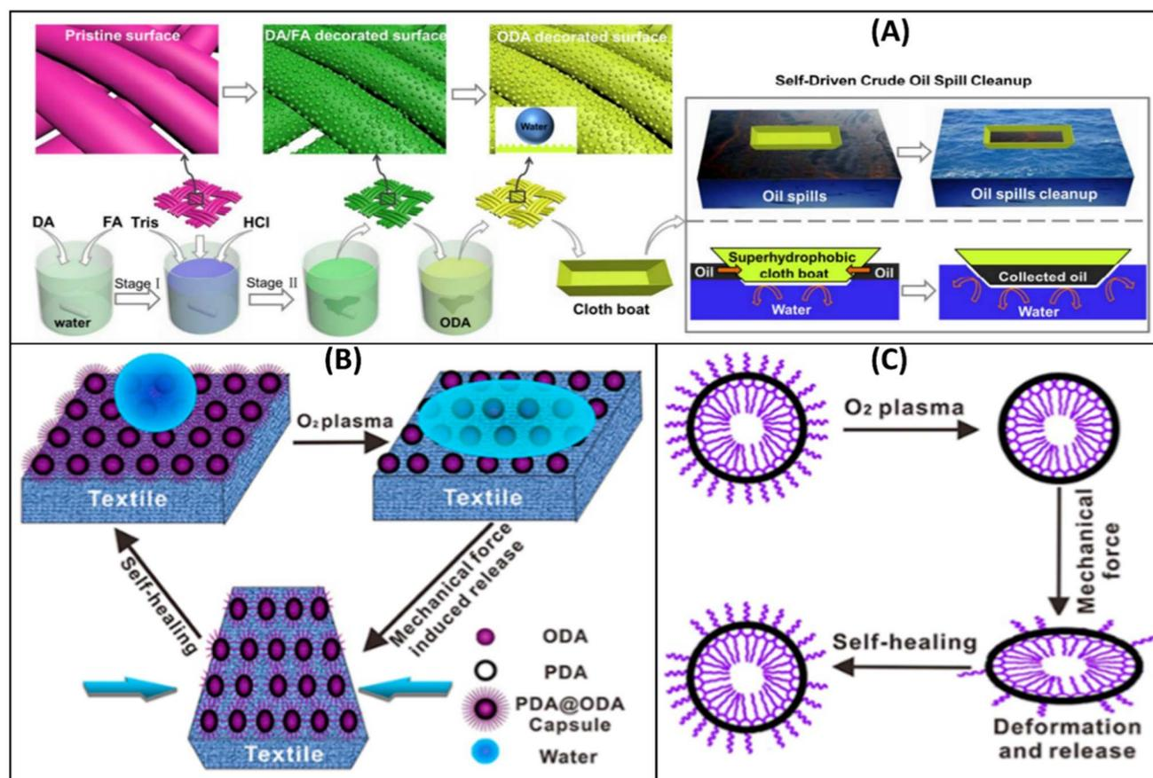
Fig. 3 Schematic illustration of the fabrication of a superhydrophobic fabric with a micro-nanostructure *via* a novel mussel-inspired approach, and a superhydrophobic cloth boat made from the fabric for self-driven oil spill cleanup (A), reproduced with permission from ref. 69. Regeneration of hydrophobicity through mechanical stimulation (B) and mechanism in the self-healing process during compression (C), reproduced with permission from ref. 70.
