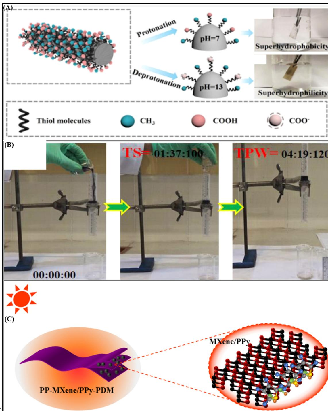
Fig. 10 (A) Mechanism illustration of the wettability switching of the pH-responsive membrane at pH 7 and 13, reproduced with permission from ref. 86; (B) oil–water separation time, reproduced with permission from ref. 89; (C) schematic illustration of the photo thermal conversion in the PP-MXene/PPy-PDM membrane, reproduced with permission from ref. 90.
