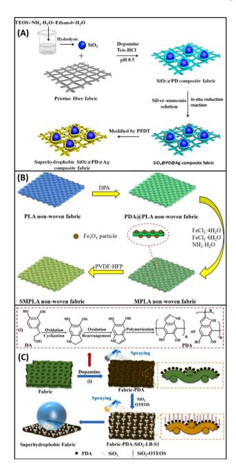
Fig. 9 Schematic illustration for the preparation of superhydrophobic fabrics (other than cotton): (A) tetra-copolyester and polypropylene/ SiO<sub>2</sub>/PD/Ag/PFDT, reproduced with permission from ref. 75; PLA/PDA/ PVDF-HFP (B), reproduced with permission from ref. 77; other materials/PDA/SiO<sub>2</sub>/OTEOS (C), reproduced with permission from ref. 82.
