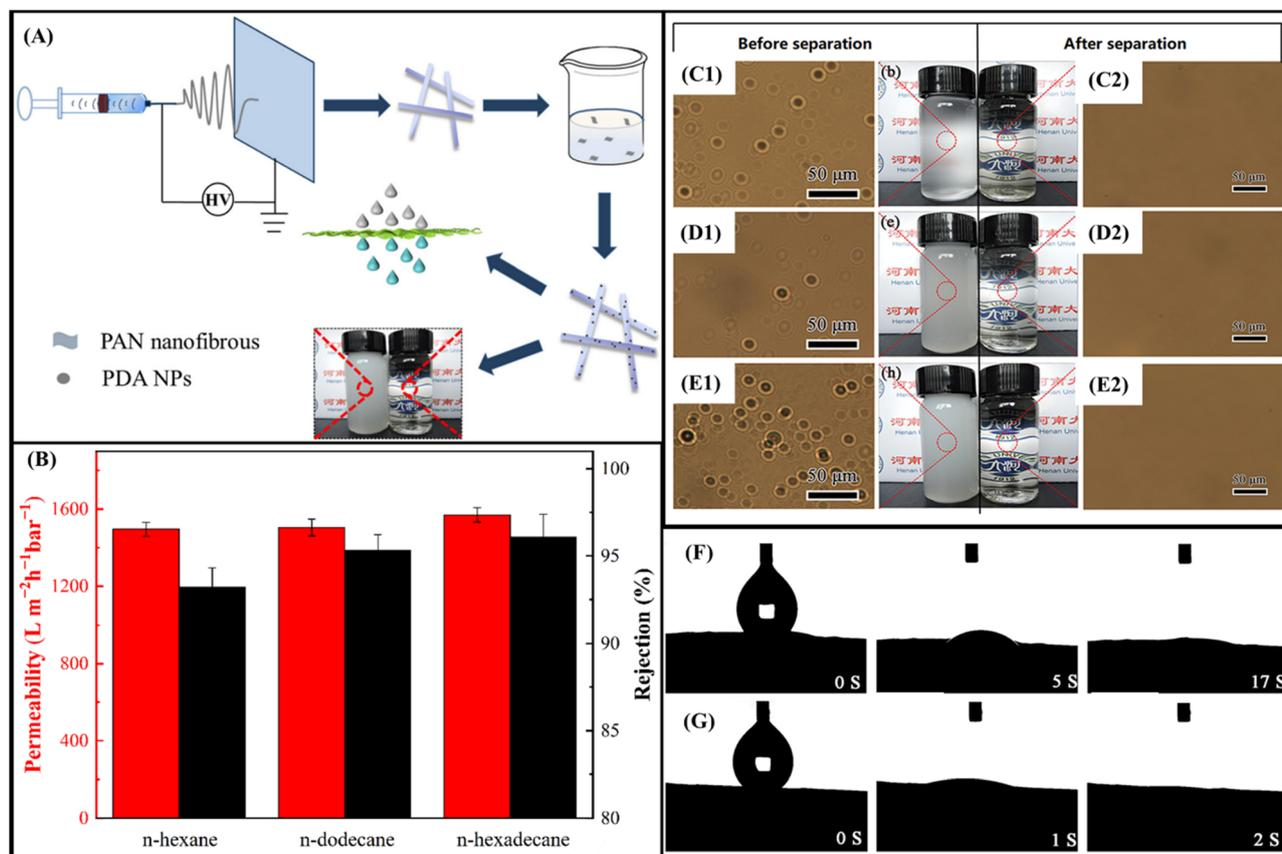
Fig. 12 Preparation process (A); permeability and separation efficiency (B); optical micrographs of *n*-hexane/water (C1), dodecane/water (D1), hexadecane/water (E1) emulsions and their separations (C2, D2, and E2) respectively; and spreading time of water drop on pristine PAN (F) and PAN@PDA (G), reproduced with permission from ref. 121.
