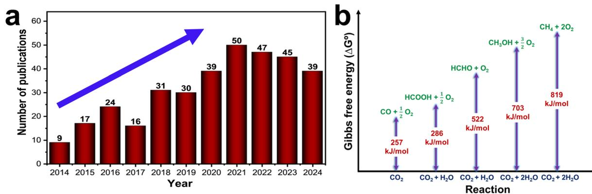
Fig. 2 (a) Publication trends (2014–2024) on Scopus for the keywords “photocatalytic reduction”, “graphene”, and “CO<sub>2</sub>”. (b) Gibbs free energy diagram of CO<sub>2</sub> photocatalytic reduction into different value-added products.
