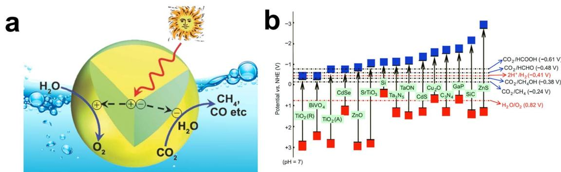
Fig. 3 (a) Schematic of the photocatalytic reduction of CO<sub>2</sub> in an aqueous medium over a graphene-based photocatalyst. Reproduced with permission from ref. 34, copyright 2014, Wiley. (b) Redox potential and band position of different semiconductors for CO<sub>2</sub> reduction into value-added products in aqueous medium. Reproduced with permission from ref. 45, copyright 2014, Springer Nature.
