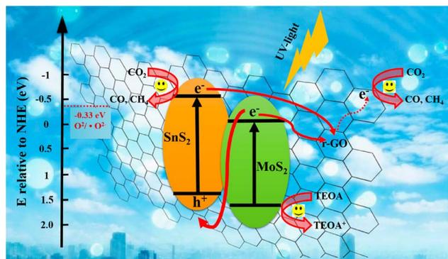
Fig. 7 A plausible mechanism of the energy band structure and charge separation over MoS<sub>2</sub>/SnS<sub>2</sub>/r-GO during photocatalytic reduction of CO<sub>2</sub>. Reproduced with permission from ref. 85, copyright 2019, the American Chemical Society.
