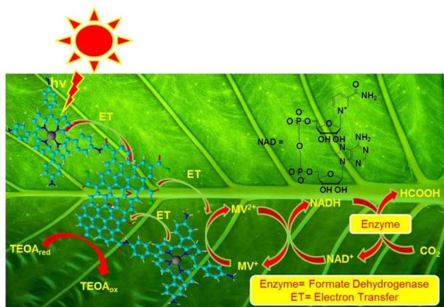
Fig. 9 Plausible pathway for the conversion of  $\text{CO}_2$  into formic acid over graphene oxide modified cobalt metallated aminoporphyrin. Reproduced with permission from ref. 67, copyright 2018, Elsevier Ltd.
