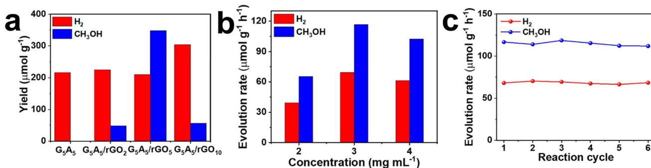
Fig. 5 (a) Hydrogen and methanol yields using G<sub>5</sub>A<sub>5</sub> and its rGO composites, (b) hydrogen and methanol yields at varying concentrations using G<sub>5</sub>A<sub>5</sub> and its rGO composites, and (c) hydrogen and methanol evolution rates using G<sub>5</sub>A<sub>5</sub>/rGO<sub>5</sub> (3 mg mL<sup>-1</sup>) under 12 h solar light. Reproduced with permission from ref. 74, copyright 2022, Elsevier Ltd.
