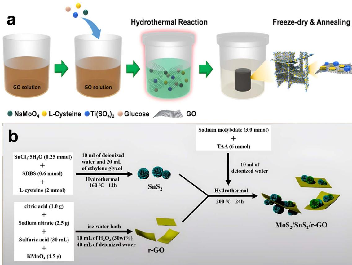
Fig. 6 (a) Illustration of the synthesis approach of a TiO<sub>2</sub>-graphene-MoS<sub>2</sub> composite. Reproduced with permission from ref. 89, copyright 2018, the American Chemical Society. (b) Schematic of the MoS<sub>2</sub>/SnS<sub>2</sub>/r-GO fabrication procedure. Reproduced with permission from ref. 85, copyright 2019, the American Chemical Society.
