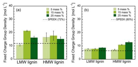
Fig. 4 Fixed group charge density for (a) SPEEK(72%) based nanocomposite membranes and (b) SPEEK(80%) based nanocomposite membranes. The dashed lines represent the average equilibrium water uptake and ion exchange capacity of neat SPEEK samples. Note, the error bars represent the standard deviation of the calculated averaged from measurements on at least three independent membranes.
