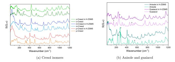
Fig. 3 INS spectra (a) p-cresol, m-cresol and o-cresol and (b) guaiacol and anisole, each as a pure compound, and then when loaded into H-ZSM-5. Example bands exhibiting more notable changes when dosed into the zeolite have been identified (\*).
