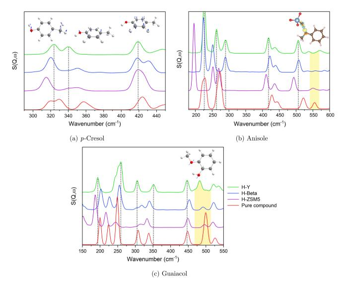
Fig. 11 Simulated spectra of *p*-cresol, anisole and guaiacol in zeolites HY, H-Beta, and H-ZSM-5 compared to the pure compounds. For (b) and (c), the bands attributed to the methoxy bend are highlighted in yellow.
