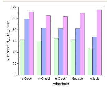
Fig. 6 The number of  $H_{ads}$ – $O_{zeo}$  pairs within 5 Å of one another, supporting the hypothesis of a stabilising confinement effect of zeolite HY (green), H-Beta (blue), and H-ZSM-5 (purple).
