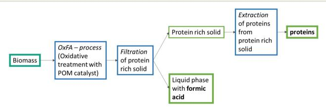
Fig. 1 Schematic flow-chart of the ProFA process. The unit operations are marked in blue and the reactants and products are colored greenish.
