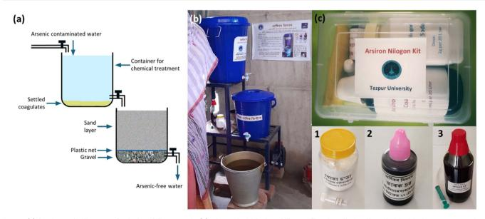
Fig. 4 (a) A schematic diagram of a Arsiron Nilogon unit; (b) a household Arsiron Nilogon filter installed at Kuruabahi with the upper container serving as a coagulation–sedimentation chamber, while the lower container is a sand-gravel filter; (c) a chemical kit which includes a bottle of  $500 \text{ g NaHCO}_3$  (1) with a small measuring cup marked for 4 g for dispensing, a dropping bottle of 5% aq. KMnO<sub>4</sub> (2) and a 500 mL bottle of 25% aq. FeCl<sub>3</sub> (3).
