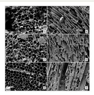
Fig. 1 SEM images of Cannabis sativa L. chemotype II stem-derived biochar produced at 400  $^{\circ}$ C (A and B), 600  $^{\circ}$ C (C and D), and 800  $^{\circ}$ C (E and F). Cross-sectional views are displayed on the left side, while longitudinal sections are shown on the right side.
