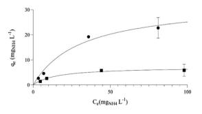
Fig. 3 Ammonia adsorption isotherms for C-400 (circles) and C-800 (squares). The fitting lines correspond to the Langmuir isotherm (with  $Q_0 = 32.6 \text{ mg}_{\text{NH4}} \text{ L}^{-1}, k_{\text{L}} = 0.032 \text{ L} \text{ mg}_{\text{NH4}}^{-1}, R^2 = 0.986 \text{ for C-400}$  and  $Q_0 = 7.1 \text{ mg}_{\text{NH4}} \text{ L}^{-1}, k_{\text{L}} = 0.065 \text{ L} \text{ mg}_{\text{NH4}}^{-1}, R^2 = 0.984, \text{ for C-800}.$
