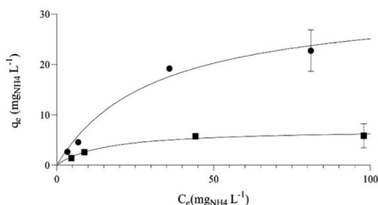
Fig. 3 Ammonia adsorption isotherms for C-400 (circles) and C-800 (squares). The fitting lines correspond to the Langmuir isotherm (with  $Q_0 = 32.6 \text{ mg}_{\text{NH}_4} \text{ L}^{-1}$ ,  $k_L = 0.032 \text{ L mg}_{\text{NH}_4}^{-1}$ ,  $R^2 = 0.986$  for C-400 and  $Q_0 = 7.1 \text{ mg}_{\text{NH}_4} \text{ L}^{-1}$ ,  $k_L = 0.065 \text{ L mg}_{\text{NH}_4}^{-1}$ ,  $R^2 = 0.984$ , for C-800).
