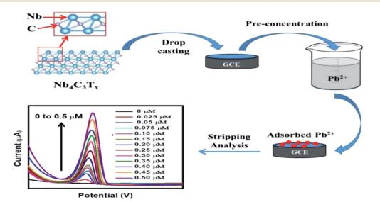
Fig. 6 Synthesis route of  $Nb_4C_3T_x/GEC$ -modified electrode for the detection of  $Pb^{2+}$  ions. Reproduced from ref. 95. Copyright (2020), adopted with permission from The Royal Chemical Society.
