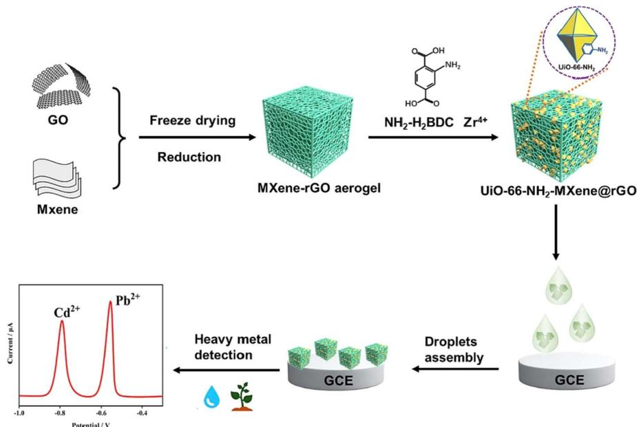
Fig. 3 Synthesis route of UiO-66-NH<sub>2</sub>-MXene@rGO/GCE-based modified sensor for the simultaneous determination of Cd<sup>2+</sup> and Pb<sup>2+</sup> ions. Reproduced from ref. 87. Copyright (2024), adopted with permission from Elsevier.
