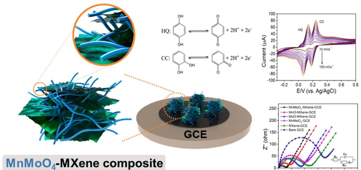
Fig. 14 Modification of the surface of GCE using the  $\text{MnMoO}_4$ -MXene nanocomposite material for the detection of hydroquinone and catechol.<sup>145</sup> Copyright, adopted from Elsevier.
