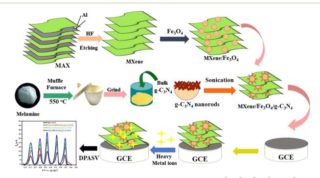
Fig. 4 Synthesis route for  $Ti_3C_2(HF)/Fe_3O_4/g-C_3N_4$  nanocomposite material and detection of  $Zn^{2+}$ ,  $Cd^{2+}$ ,  $Pb^{2+}$ ,  $Cu^{2+}$ , and  $Hg^{2+}$  ions. Reproduced from ref. 90. Copyright (2023), adopted with permission from Elsevier.
