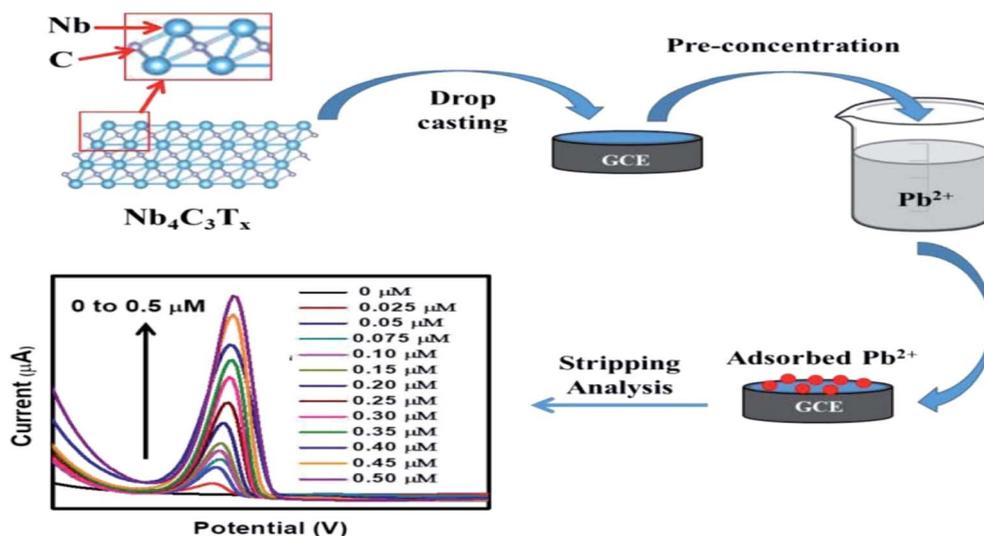
Fig. 6 Synthesis route of  $\text{Nb}_4\text{C}_3\text{T}_x/\text{GCE}$ -modified electrode for the detection of  $\text{Pb}^{2+}$  ions. Reproduced from ref. 95. Copyright (2020), adopted with permission from The Royal Chemical Society.
