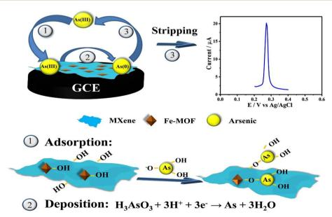
Fig. 5 Adsorption-assisted As<sup>3+</sup> ion detection on Fe-MOF/MXene/GCE by SWASV. Reproduced from ref. 92. Copyright (2022), adopted with permission from Elsevier.
