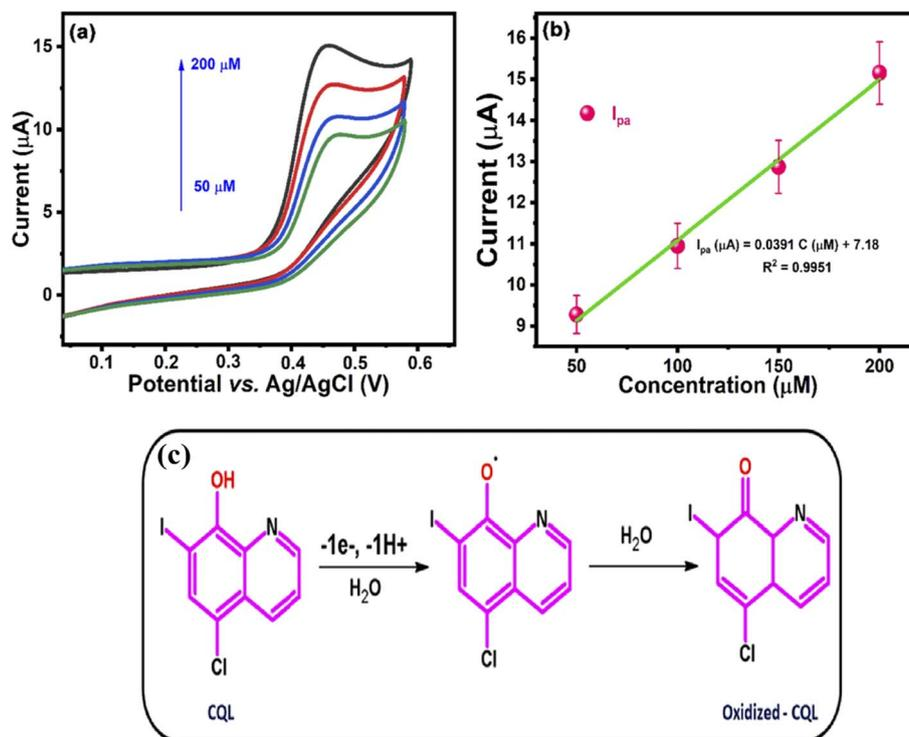
Fig. 10 (a) CVs for varying concentrations of CQL (50–200  $\mu\text{M}$ ) over the surface of VC/g-CN NSs/GCE, (b) linear plot of concentration vs. current, and (c) electro-oxidation mechanism of clioquinol drug on the surface of VC/g-CN NSs/GCE. Reproduced from ref. 130. Copyright (2023), adopted with permission from Elsevier.
