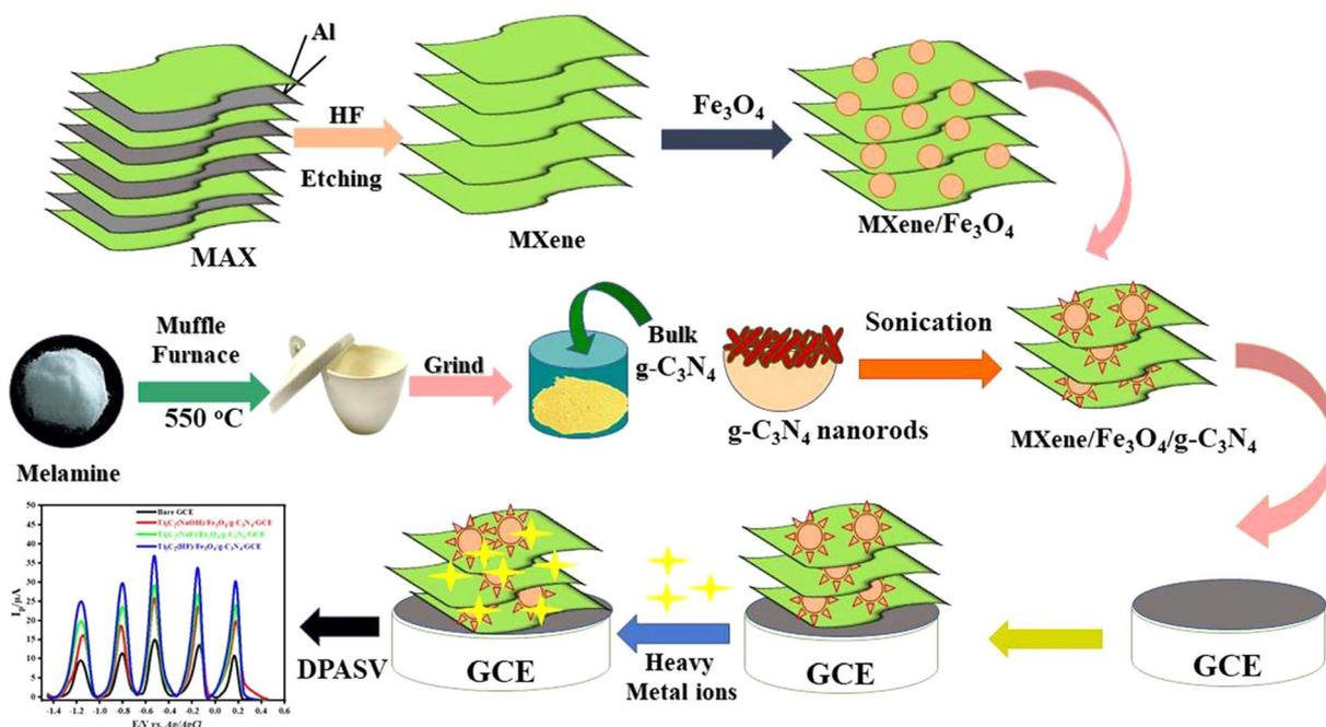
Fig. 4 Synthesis route for Ti<sub>3</sub>C<sub>2</sub>(HF)/Fe<sub>3</sub>O<sub>4</sub>/g-C<sub>3</sub>N<sub>4</sub> nanocomposite material and detection of Zn<sup>2+</sup>, Cd<sup>2+</sup>, Pb<sup>2+</sup>, Cu<sup>2+</sup>, and Hg<sup>2+</sup> ions. Reproduced from ref. 90. Copyright (2023), adopted with permission from Elsevier.
