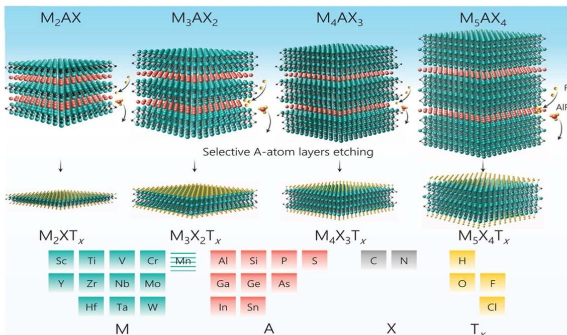
Fig. 1 MAX phases used for the synthesis of different MXene forms.<sup>71</sup> Copyright (2021), adopted from John Wiley and Sons.
