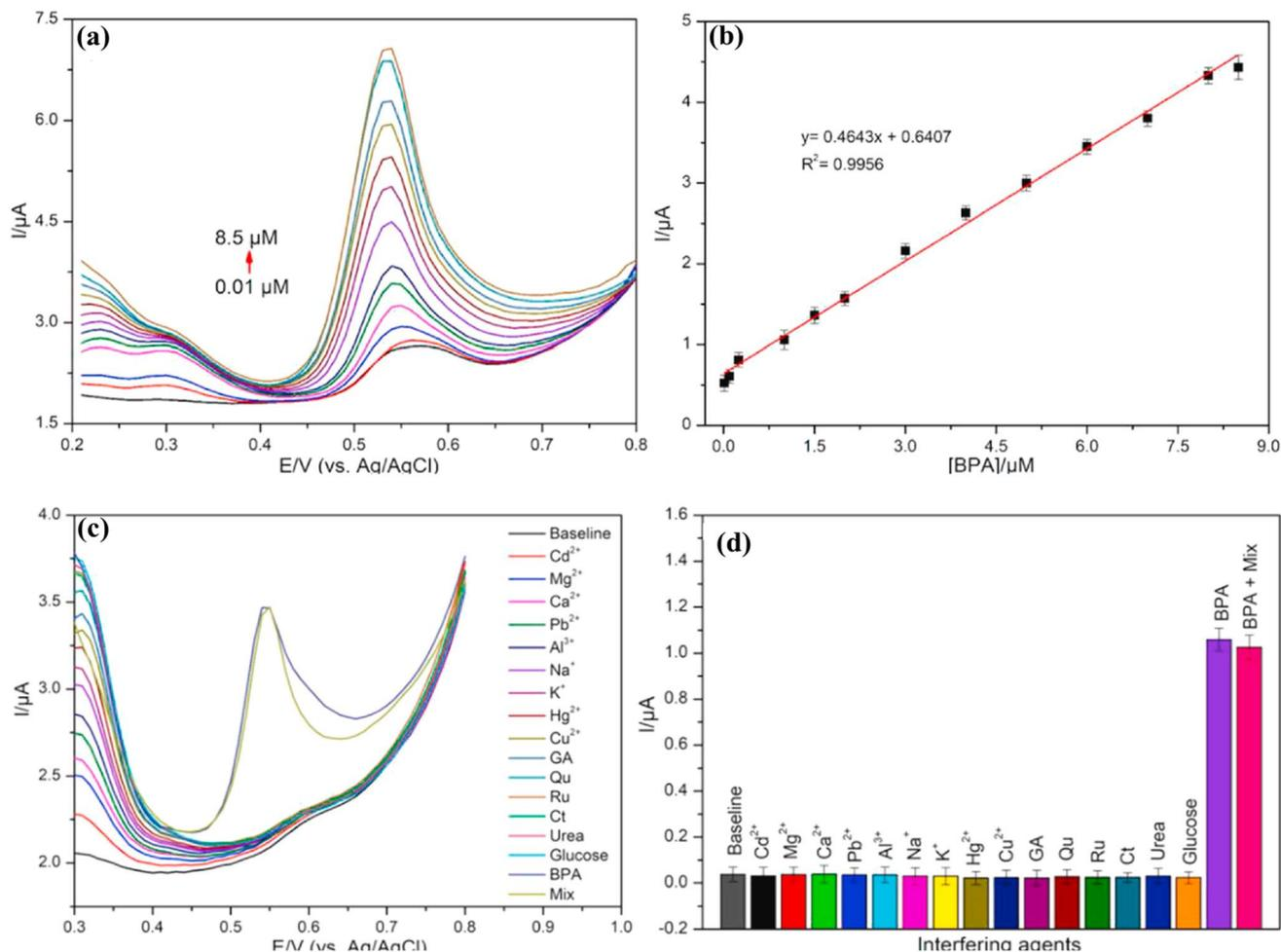
Fig. 12 (a) DPV responses at different concentrations of BPA on  $\text{Mo}_2\text{Ti}_2\text{AlC}_3/\text{MWCNT}/\text{GCE}$  and (b) the linear relationship between current and concentration of BPA. (c and d) Selective determination of BPA. Reproduced from ref. 141. Copyright (2022), adopted with permission from Elsevier.
