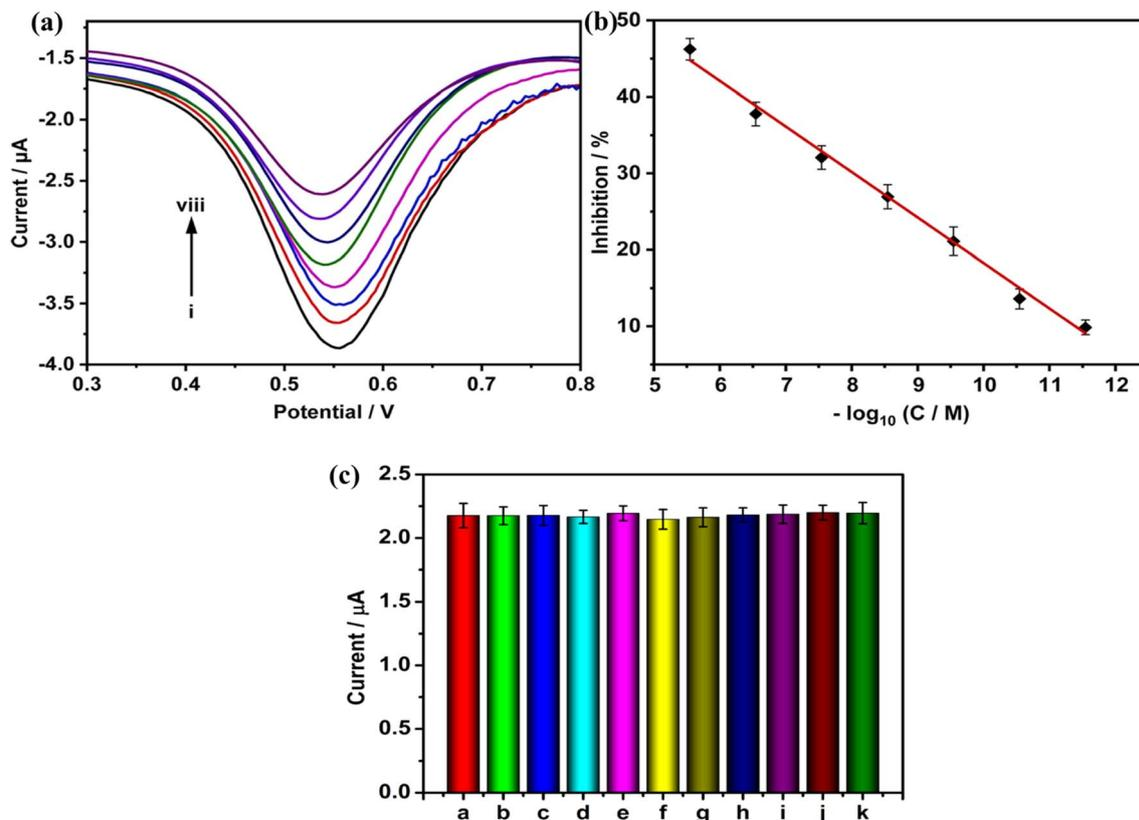
Fig. 8 (a and b) DPV responses of the modified electrode and (c) effect of foreign interferent species in the determination of chlorpyrifos pesticide. Reproduced from ref. 110. Copyright (2022), adopted with permission from Elsevier.
