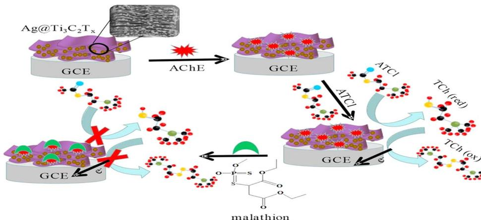
Fig. 7 Synthesis route of Ag@Ti<sub>3</sub>C<sub>2</sub>T<sub>x</sub> for the detection of the organophosphate pesticide malathion. Reproduced from ref. 106. Copyright (2018), adopted with permission from Elsevier.
